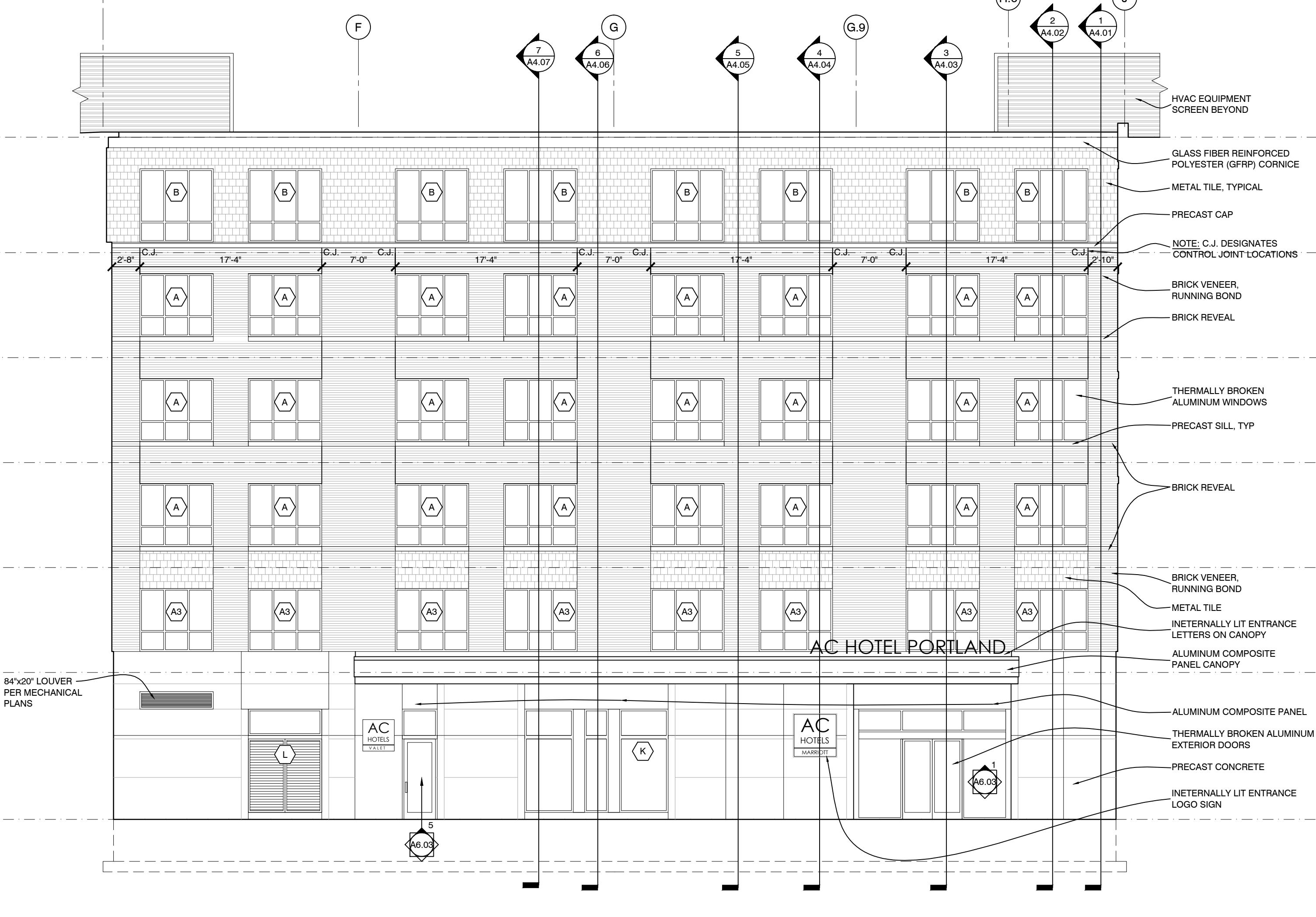
1 SOUTH EXTERIOR ELEVATION 1/8" = 1'-0"
