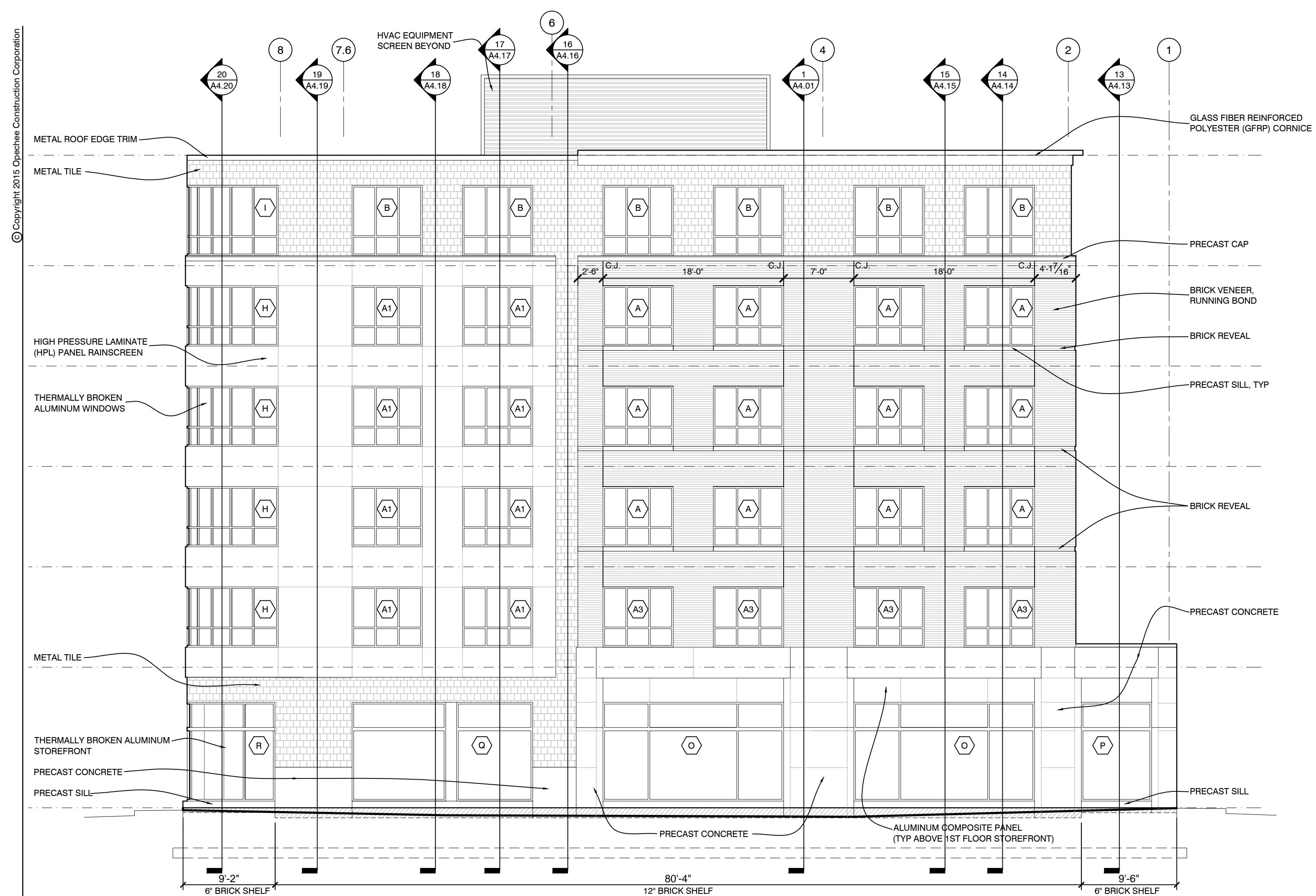
5 WEST EXTERIOR ELEVATION 1/8" = 1'-0"
