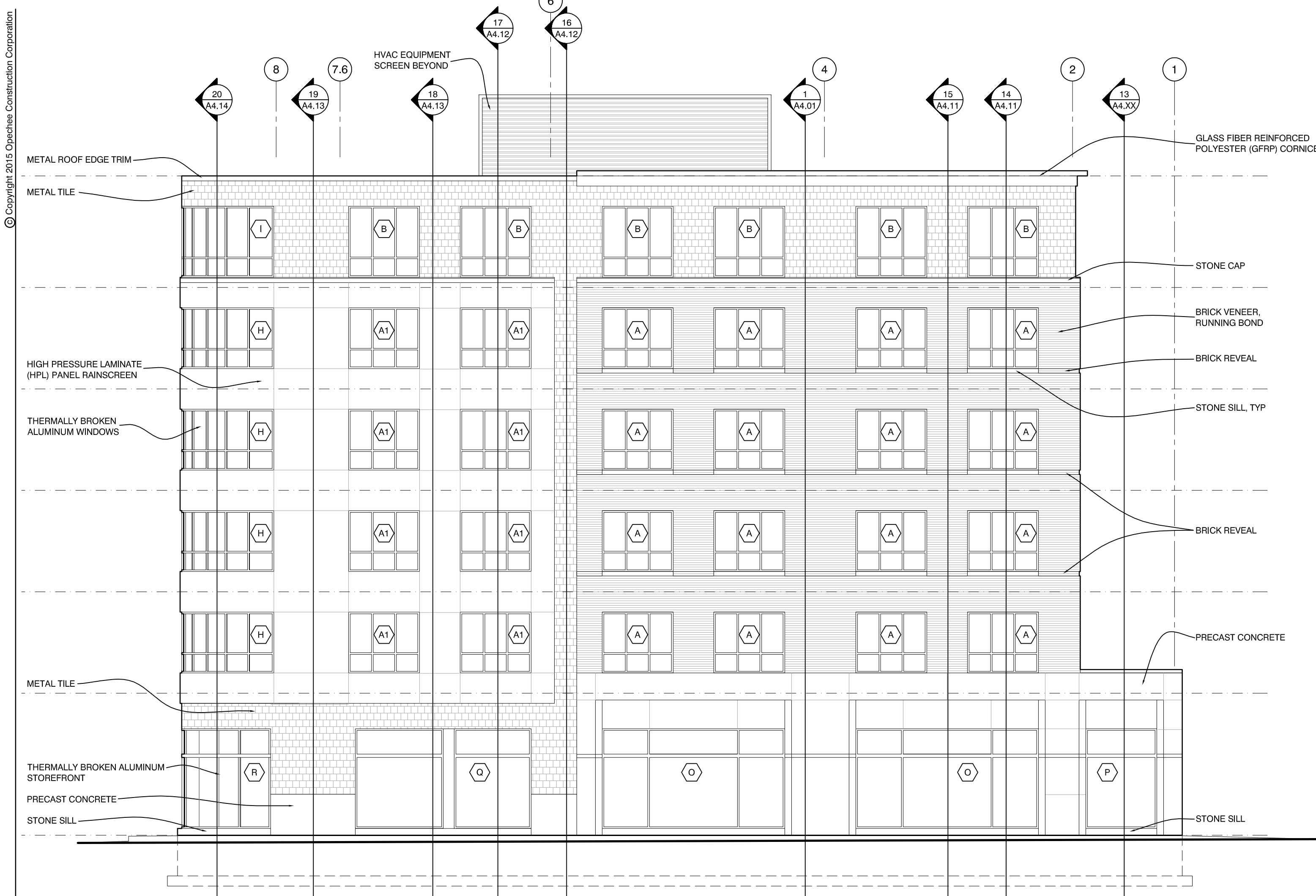
5 WEST EXTERIOR ELEVATION 1/8" = 1'-0"
