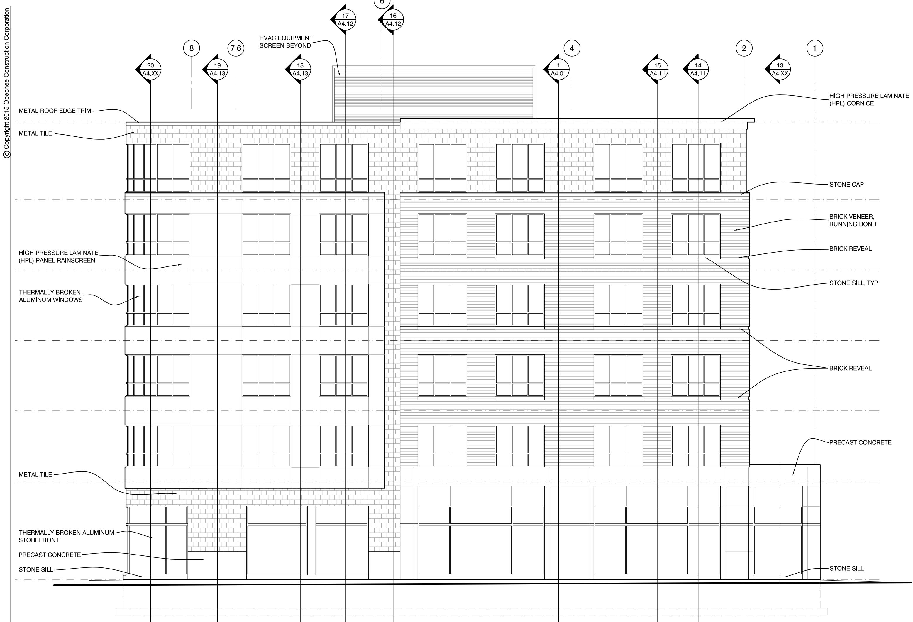
5 WEST EXTERIOR ELEVATION 1/8" = 1'-0"
