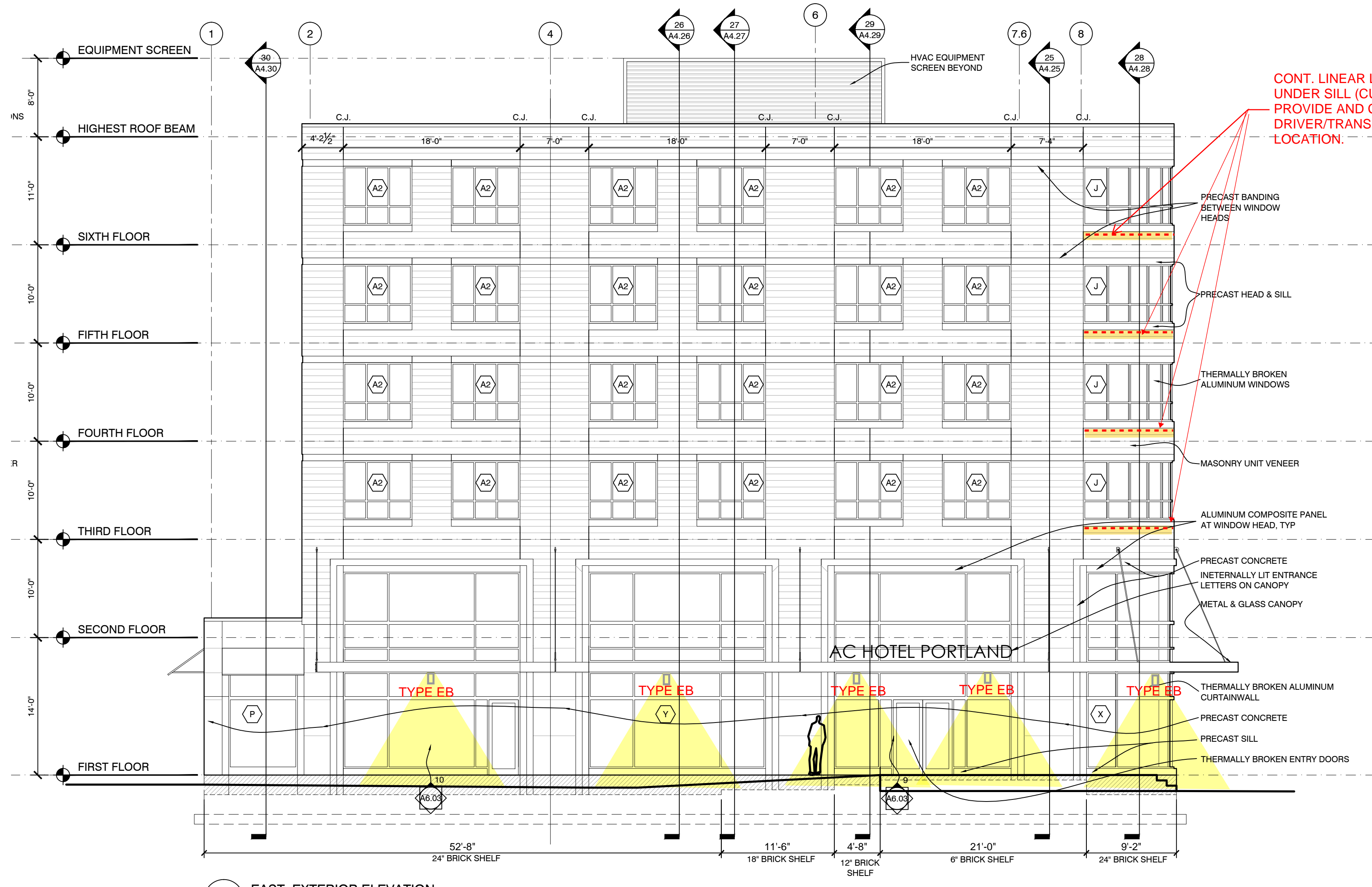
7 EAST EXTERIOR ELEVATION 1/8" = 1'-0"
