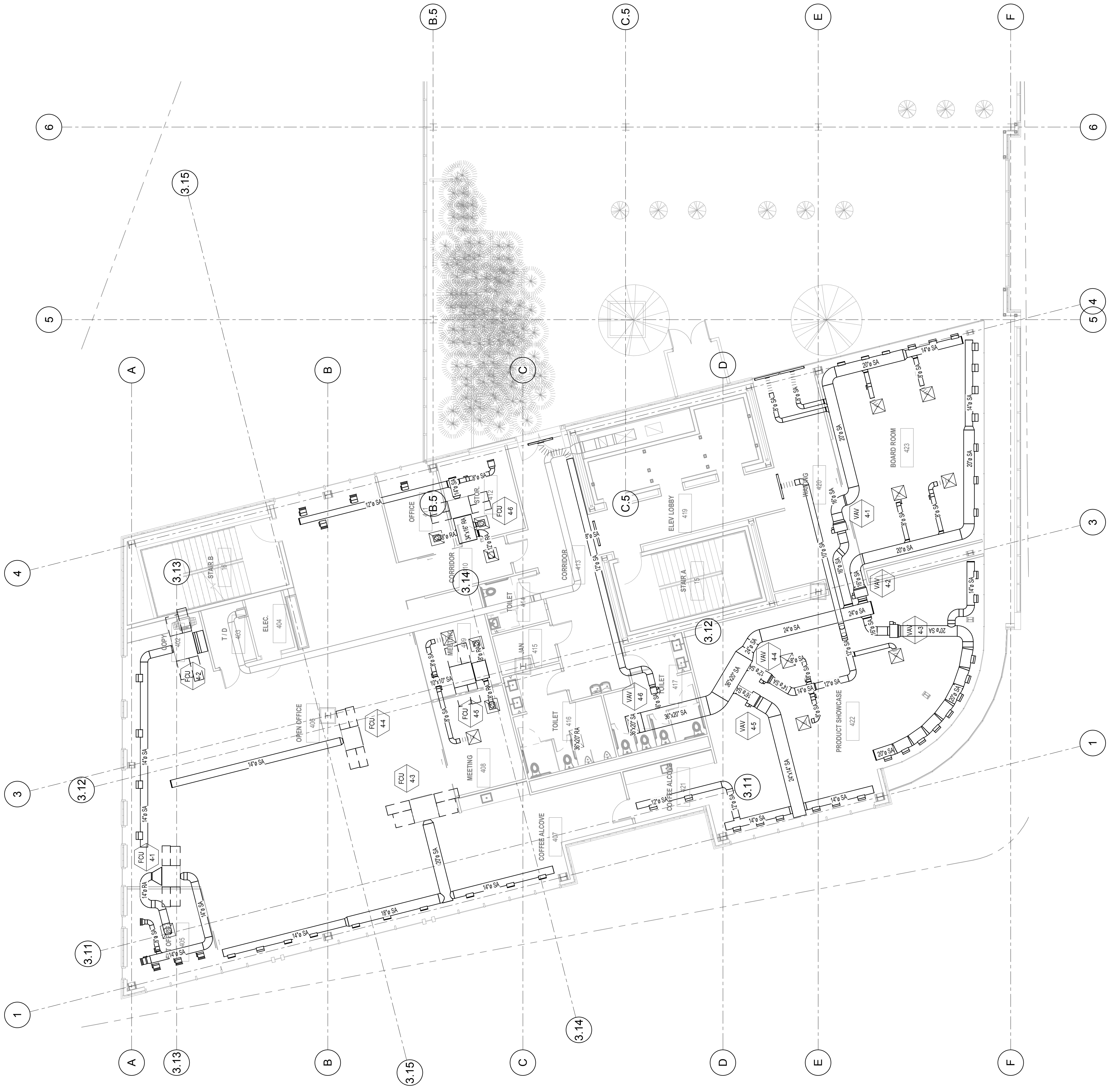
① 4TH FLOOR HVAC DUCTWORK PLAN A 1/8" = 1'-0"
