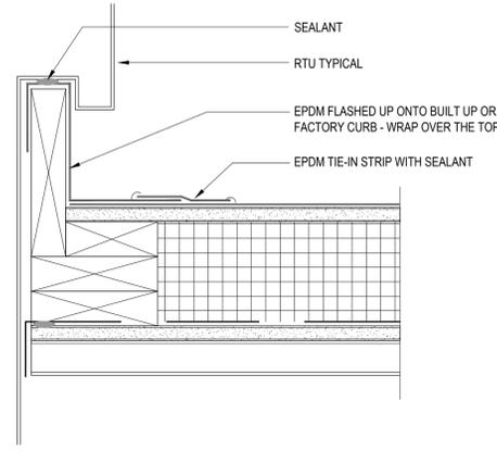
**4 MECHANICAL CURB ROOF FLASHING**
