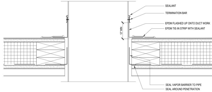
**3 MECHANICAL DUCT FLASHING AT ROOF PENETRATION**
