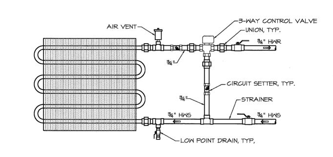
VAV HM COIL PIPING DETAIL (\\-|46 \ \\-|43) SCALE: NONE
