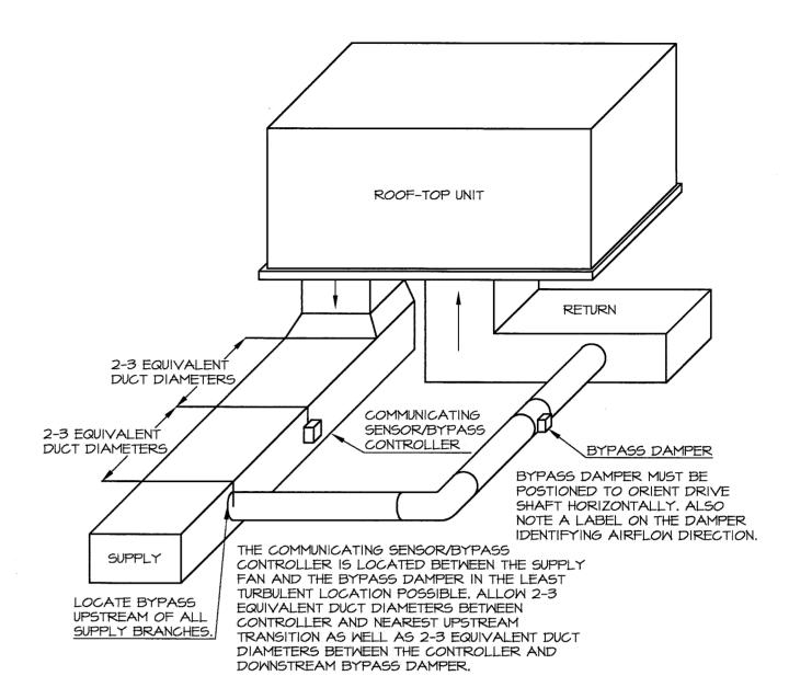
COMMUNICATING SENSOR/BYPASS CONTROL \$ BYPASS DAMPER INSTALLATION DETAIL
