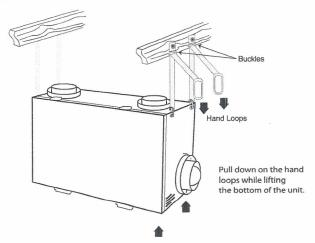
4. Make certain the unit is level. Adjust the unit down by lifting up on the buckle. Fold the hand loops and excess strap and secure with a nylon tie.
