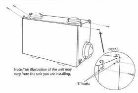
3. Hook the bottom grommets of the straps through the "S" hooks. Pull down on the hand loops while lifting up the bottom of the unit. Repeat at opposite end of the unit.
