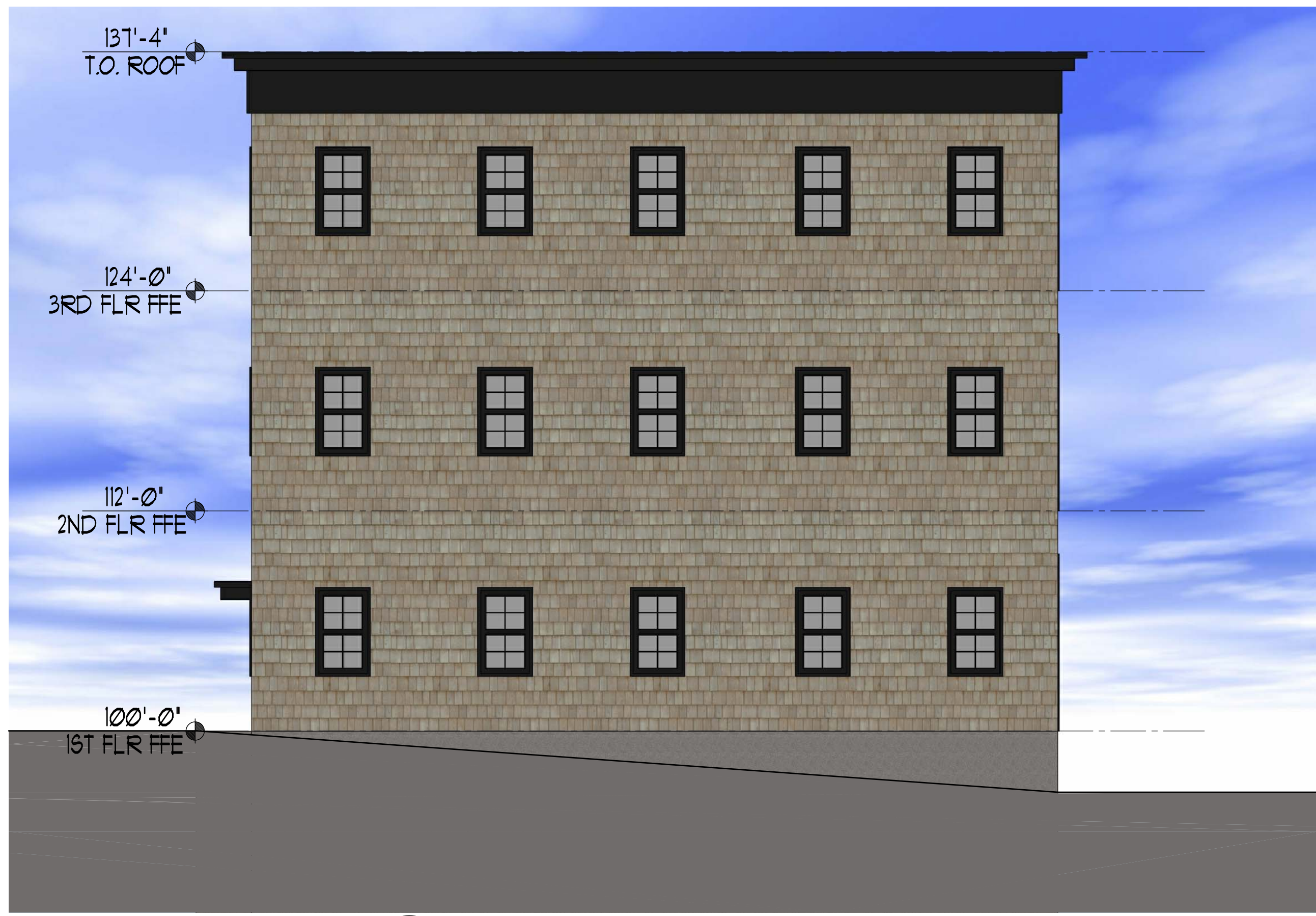
4 ELEVATION - REAR SCALE: 3/16" = 1'-0"
