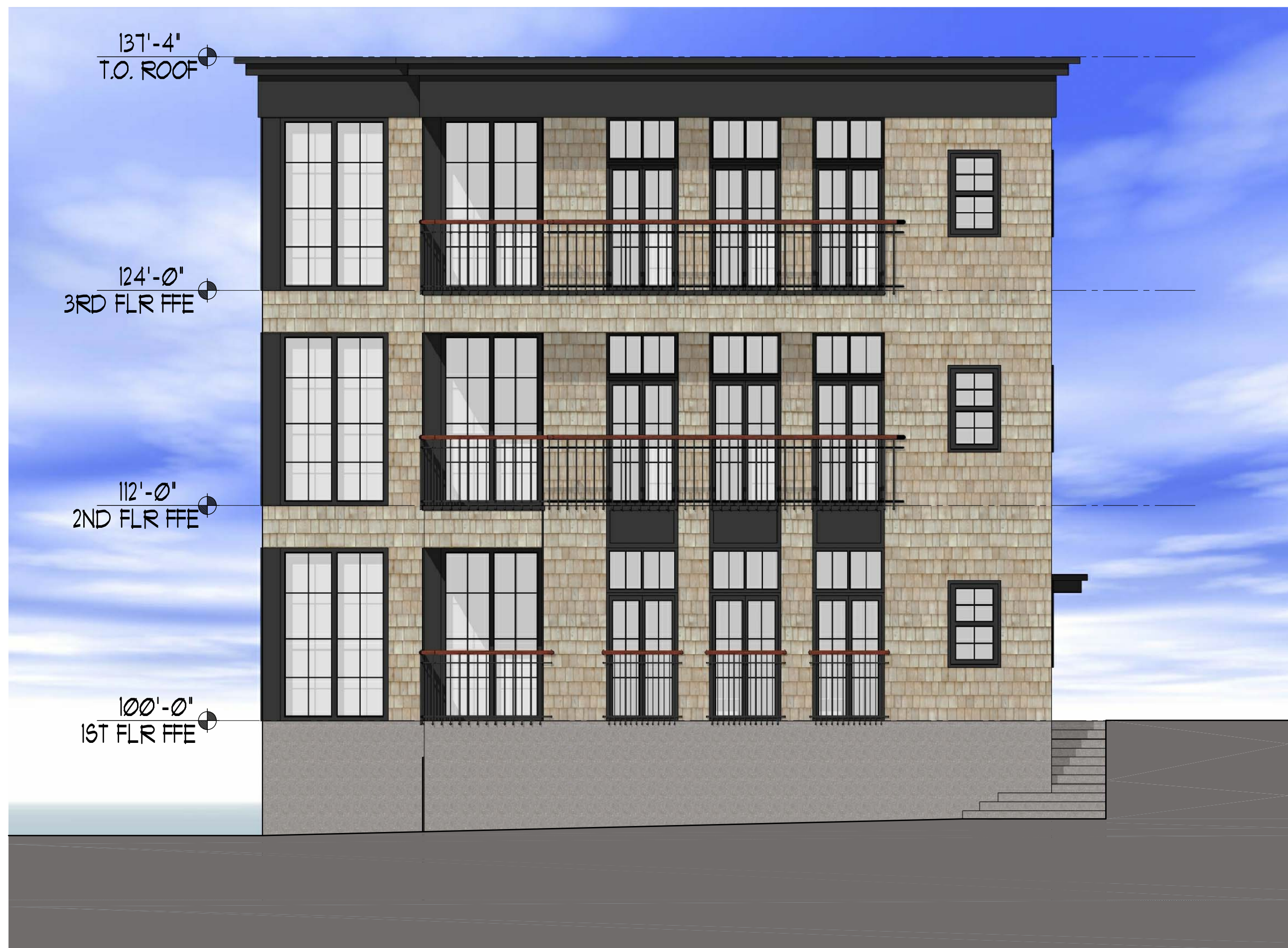
3 ELEVATION - FRONT - FORE ST SCALE: 3/16" = 1'-0"
