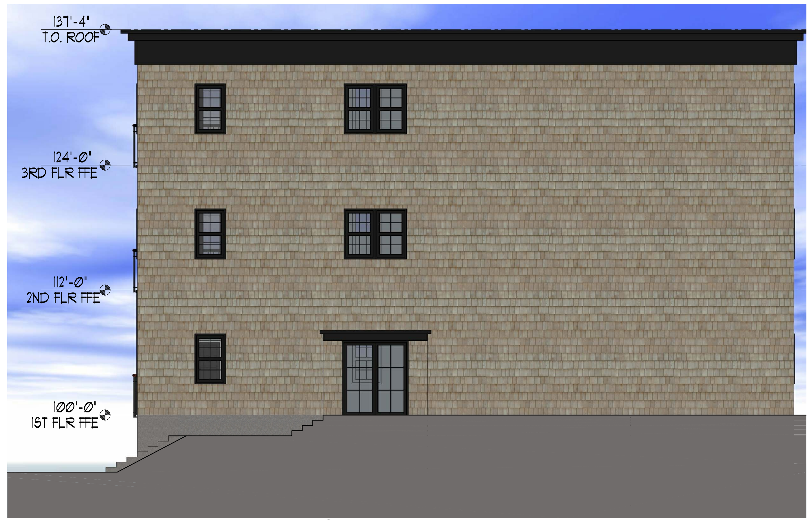
2 ELEVATION - SIDE SCALE: 3/16" = 1'-0"
