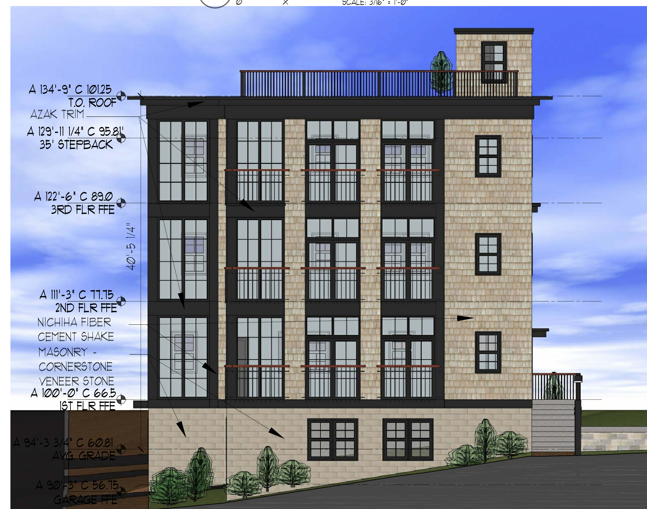
3 ELEVATION - FRONT - FORE ST
