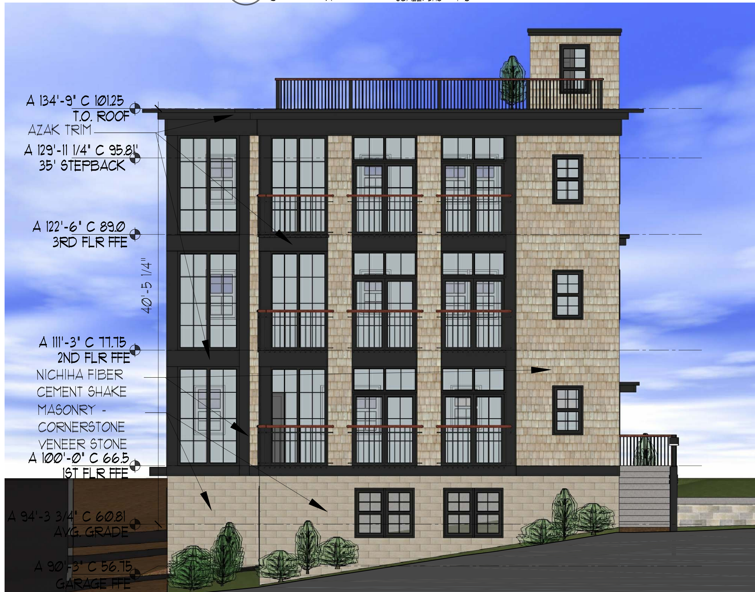
3 ELEVATION - FRONT - FORE ST
