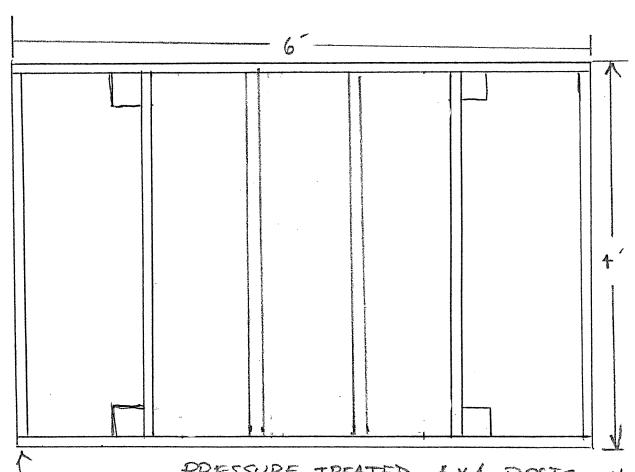
PRESSURE TREATED + X4 POSTS ON CONCRETE
