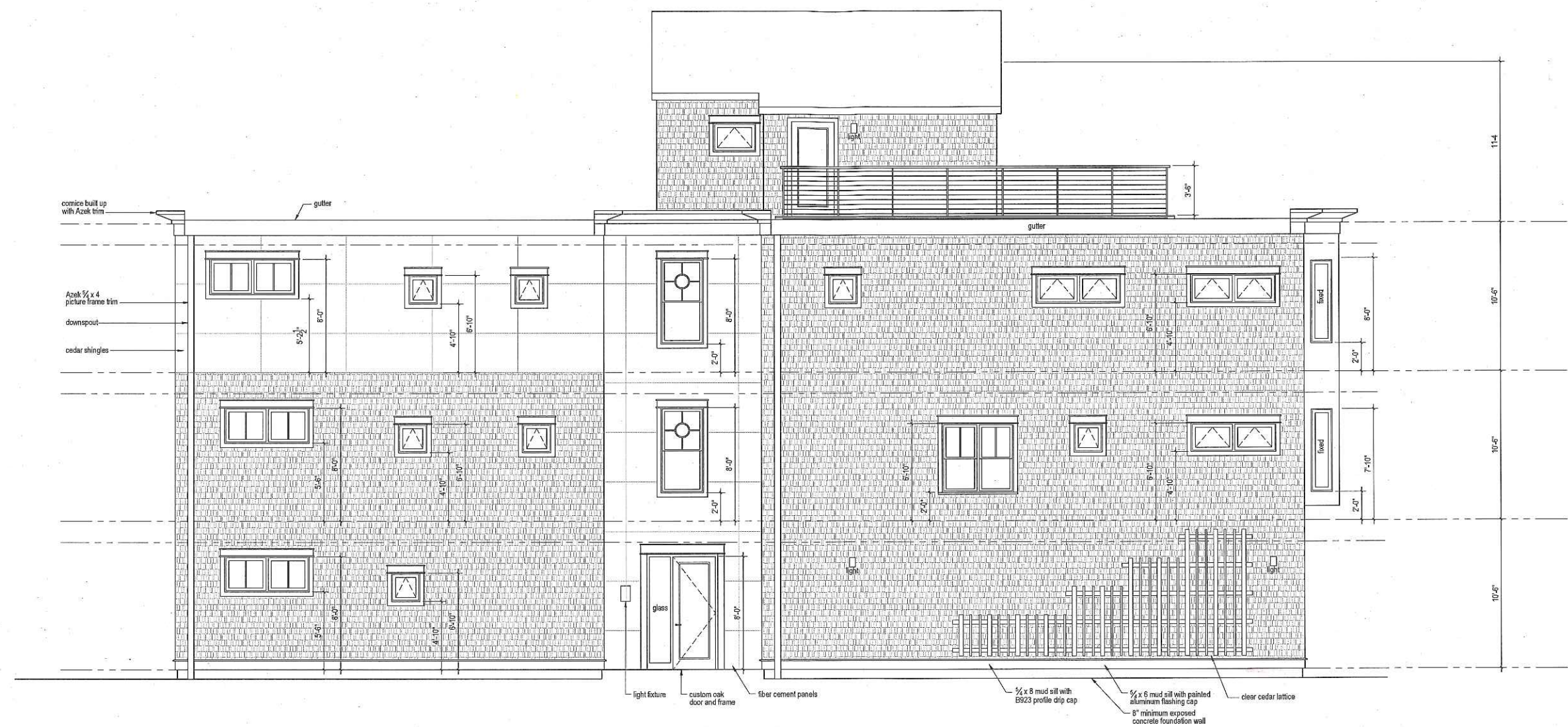
2 Side (North) Elevation. 1/4" = 1'-0"
