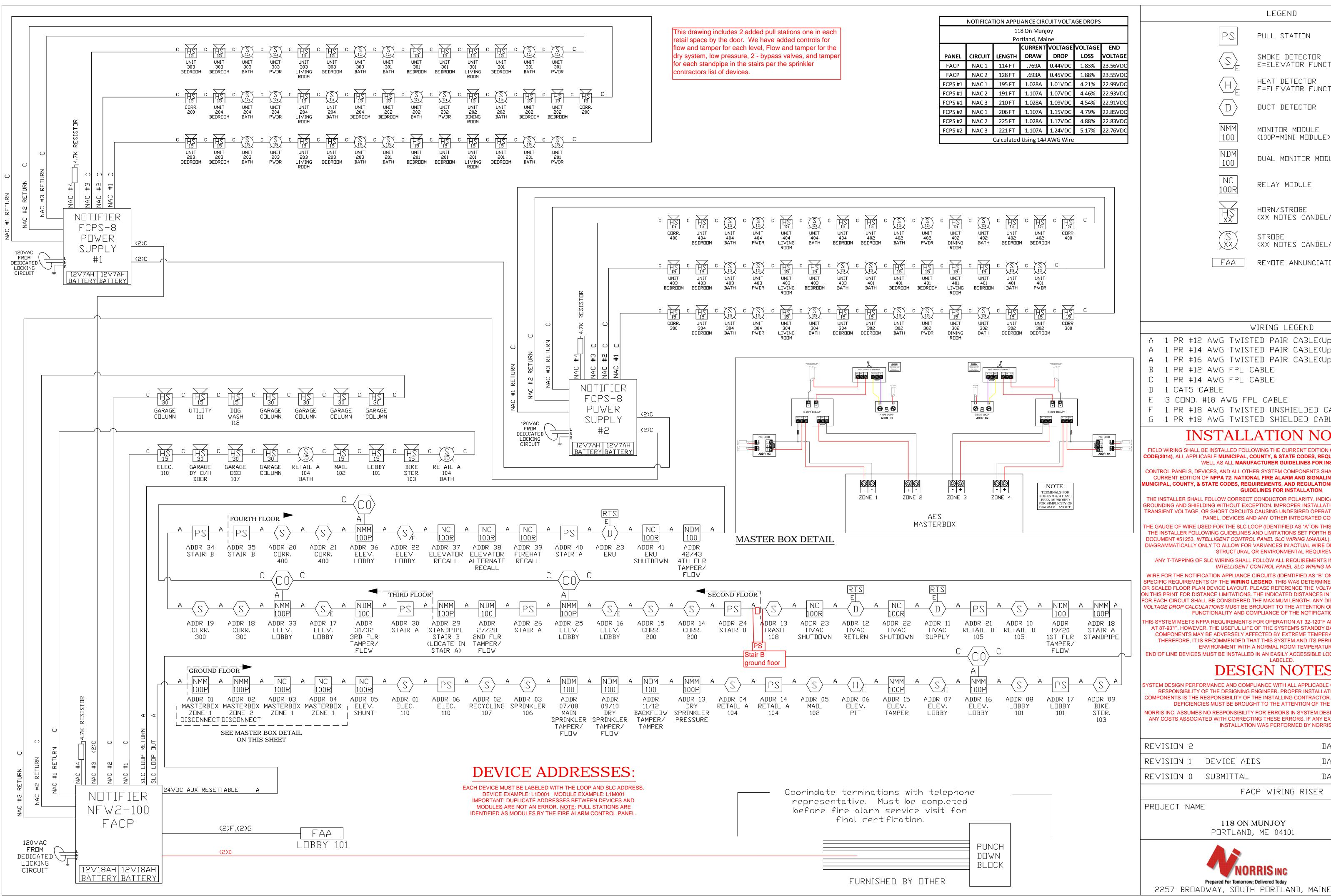
LEGEND PULL STATION SMOKE DETECTOR E=ELEVATOR FUNCTION HEAT DETECTOR E=ELEVATOR FUNCTION DUCT DETECTOR MONITOR MODULE (100P=MINI MODULE) DUAL MONITOR MODULE RELAY MODULE HORN/STROBE (XX NOTES CANDELA)
