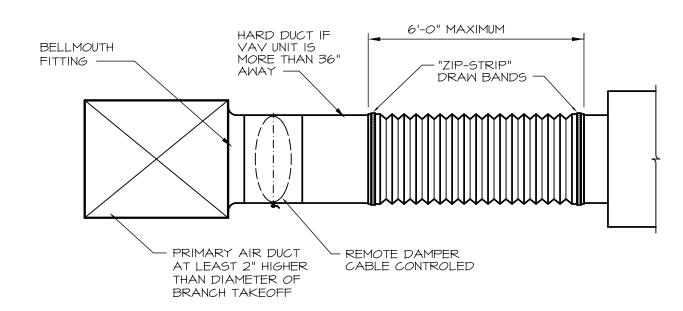
FLEXIBLE DUCT CONNECTION TO SUPPLY OUTLET NO SCALE
