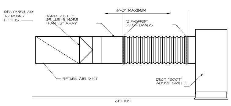
FLEXIBLE DUCT & RETURN GRILLE CONNECTION NO SCALE
