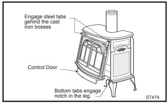
Fig. 53 Install the front plate.
