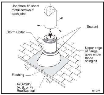
Fig. 32 Roof support and flashing.
