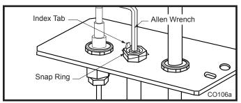
Fig. 77 Remove pilot orifice.
