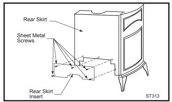
Fig. 15 Remove rear skirt insert.
