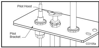
Fig. 78 Remove pilot hood.
