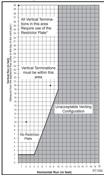
Fig. 8 Vertical vent termination window.
