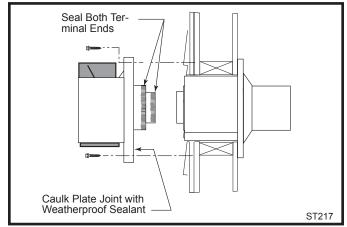
Fig. 28 Install the vent terminal.
