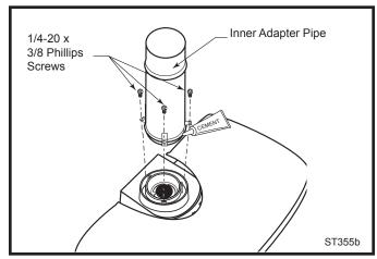
Fig. 21 Simpson Dura-Vent - install inner adapter pipe.
