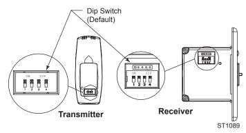
**Fig. 58** The switches on the transmitter and receiver must match.
