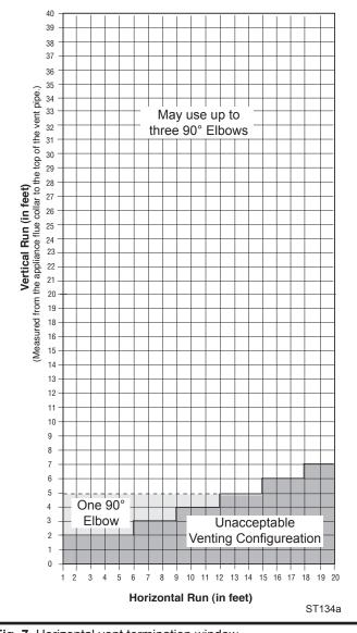
Fig. 7 Horizontal vent termination window.
