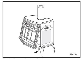
Fig. 83 Remove the stove front.
