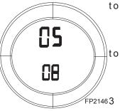
**Fig. 65** Blower time delay display.
