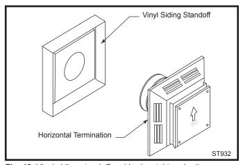
Fig. 42 Vinyl siding standoff and horizontal termination.
