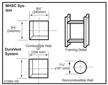
Fig. 23 Locate vent opening.
