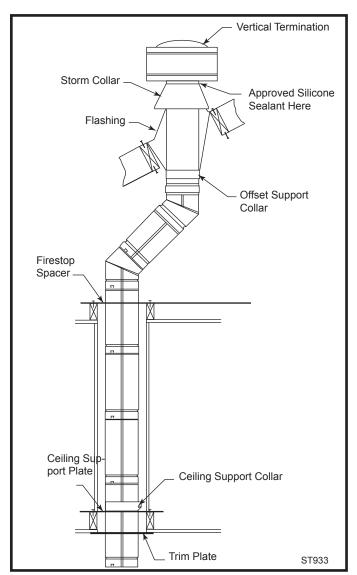
Fig. 43 Typical vertical venting configuration.
