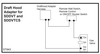
Fig. 88 Draft hood adapter wiring.
