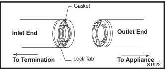
Fig. 33 Joint connection.
