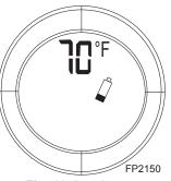
Fig. 66 Low battery display.
