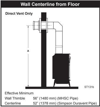
Fig. 5 Minimum wall thimble centerline.
