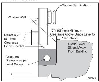
Fig. 39 Below grade installation.
