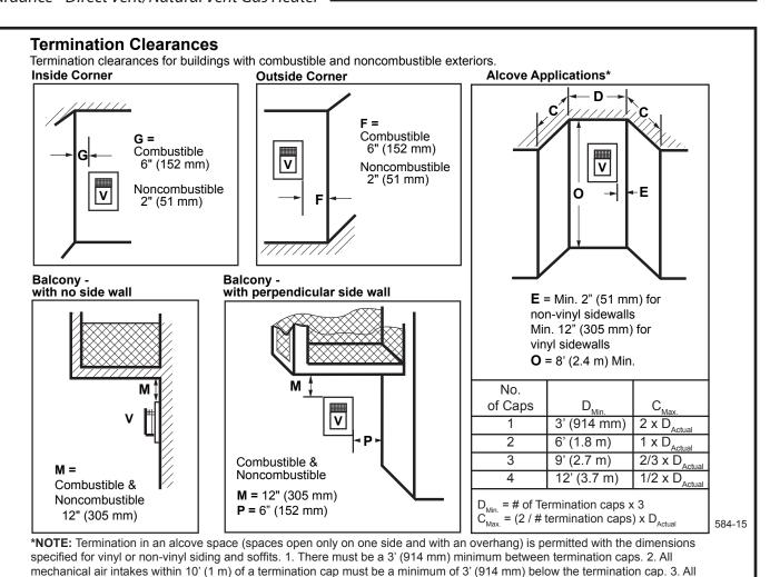
Fig. 12 Termination clearances.
