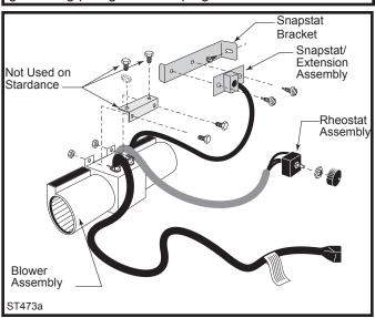
Fig. 14 Fan kit components.
