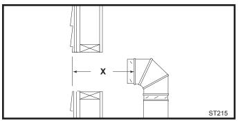
Fig. 26 Measure the horizontal length.
