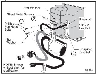
Fig. 16 Attach the fan assembly and the snapstat.
