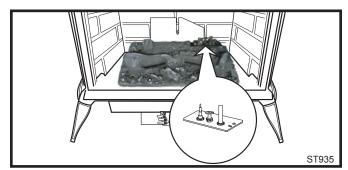
Fig. 76 Pilot assembly location.
