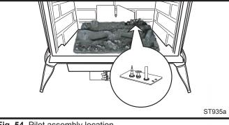
Fig. 54 Pilot assembly location.
