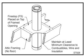
Fig. 38 Firestop spacer.
