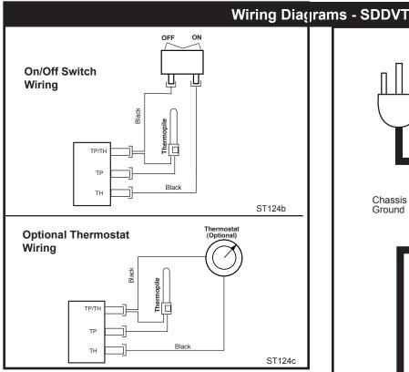
Fig. 87 On/Off switch and optional thermostat circuit.
