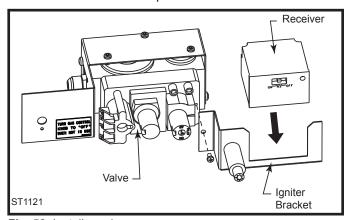
Fig. 52 Install receiver.
