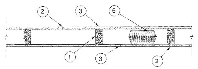
1. Wood Studs — Nom 2 by 4 in. spaced 16 in. OC max, effectively firestopped.
