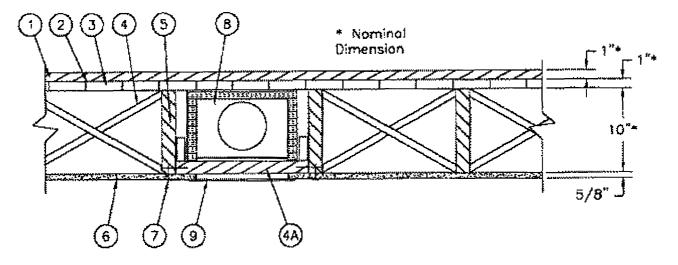
**1, 2, 3.Flooring Systems** — The finish flooring (Item 1), vapor barrier (Item 2) and the subflooring (Item 3), may consist of any one of the following systems:
