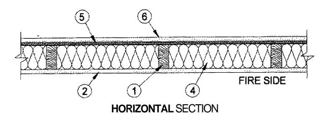
1. Wood Studs — Nom 2 by 4 in. spaced 16 in. OC with two 2 by 4 in. top and one 2 by 4 in. bottom plates. Studs laterally-braced by wood structural panel sheathing (Item 5) and effectively fire stopped at top and bottom of wall.
