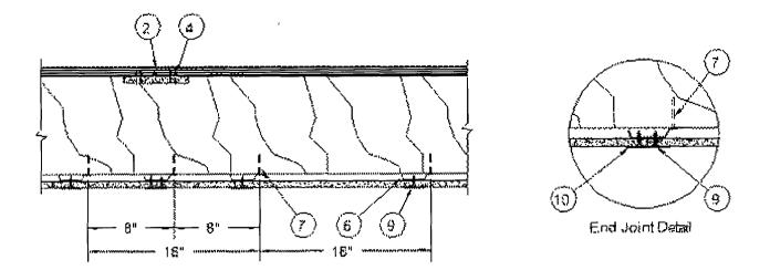
1. **Flooring** — Nom 3/4 in thick wood structural panels, min grade "Underlayment" or "Single Floor". Face grain of plywood or strength axis of panel to be perpendicular to joists with joints staggered.
