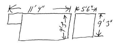
BUILD OUT OUTSIDE WALLS IN LAUNDRY ROOM 4" TO BEABLE TO INSULATE & SHEETROCK SAME All walls will be Constructed with 2X4" stude placed 16" on center attached to a 2"x4" plate on the floor and cieling. Outside walls to be insulated all walls will be then covered by 12" sheetrock, toped and pointed all work to be done inside existing walls - no outside Cordo area work required.
