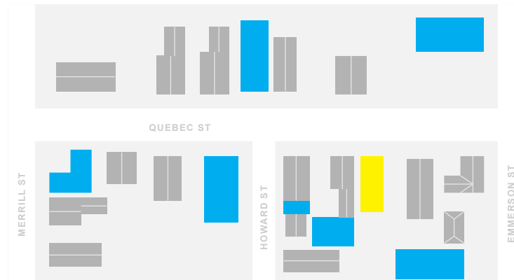
(3) Roof forms along the block are a mix of flat (blue) and sloped (gray). The proposed building site is in yellow.
