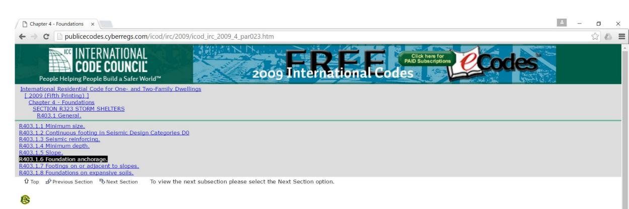
R403.1.6 Foundation anchorage. Sill plates and walls supported directly on continuous foundations shall be anchored to the foundation in accordance with this section.
