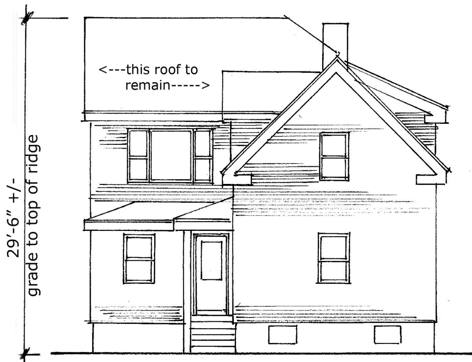
② Existing East Elevation 1/8" = 1'-0"
