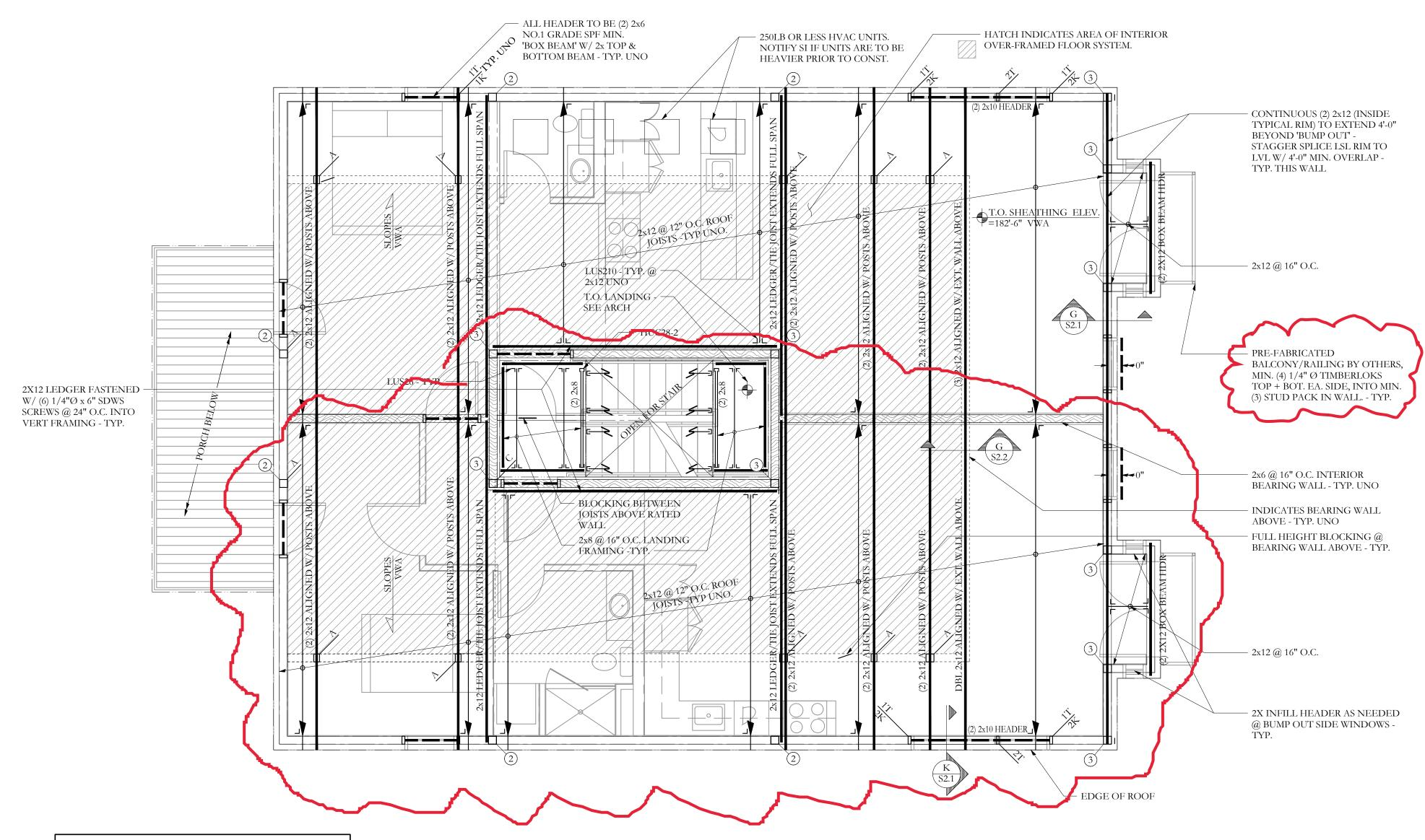
FRAMING PLAN SYMBOLS KEY WOOD POST STEEL COLUMN NUMBER OF WOOD STUDS IN POST BELOW COLUMN ABOVE THIS LEVEL COLUMN CONTINUOUS THROUGH THIS LEVEL **✓** JOIST BEARING CONTINUOUS JOIST WITH INTERMEDIATE BEARING FLUSH FRAMED JOIST BEARING WITH HANGER WOOD STUD BEARING WALL BELOW OVER FRAMING BY OTHERS -TYP NUMBER OF TRIM STUDS UNDER HEADER NUMBER OF KING STUDS ADJACENT TO HEADER
