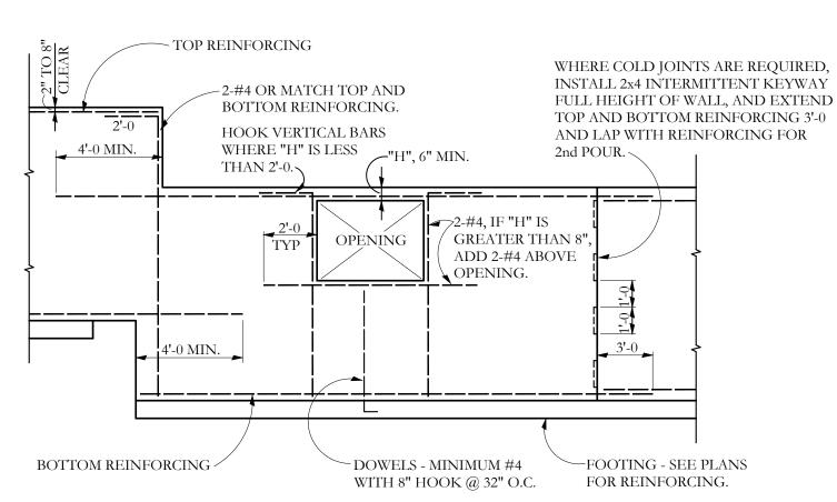
TYPICAL REINFORCING AT STEPS AND OPENINGS NO SCALE
