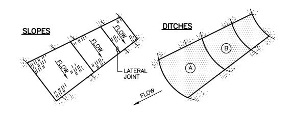
1. BURY THE TOP END OF THE MESH MATERIAL IN A 6" TRENCH AND BACKFILL AND TAMP TRENCHING SECURE END WITH STAPLES AT 6" SPACING, 4" DOWN FROM EXPOSED END.
