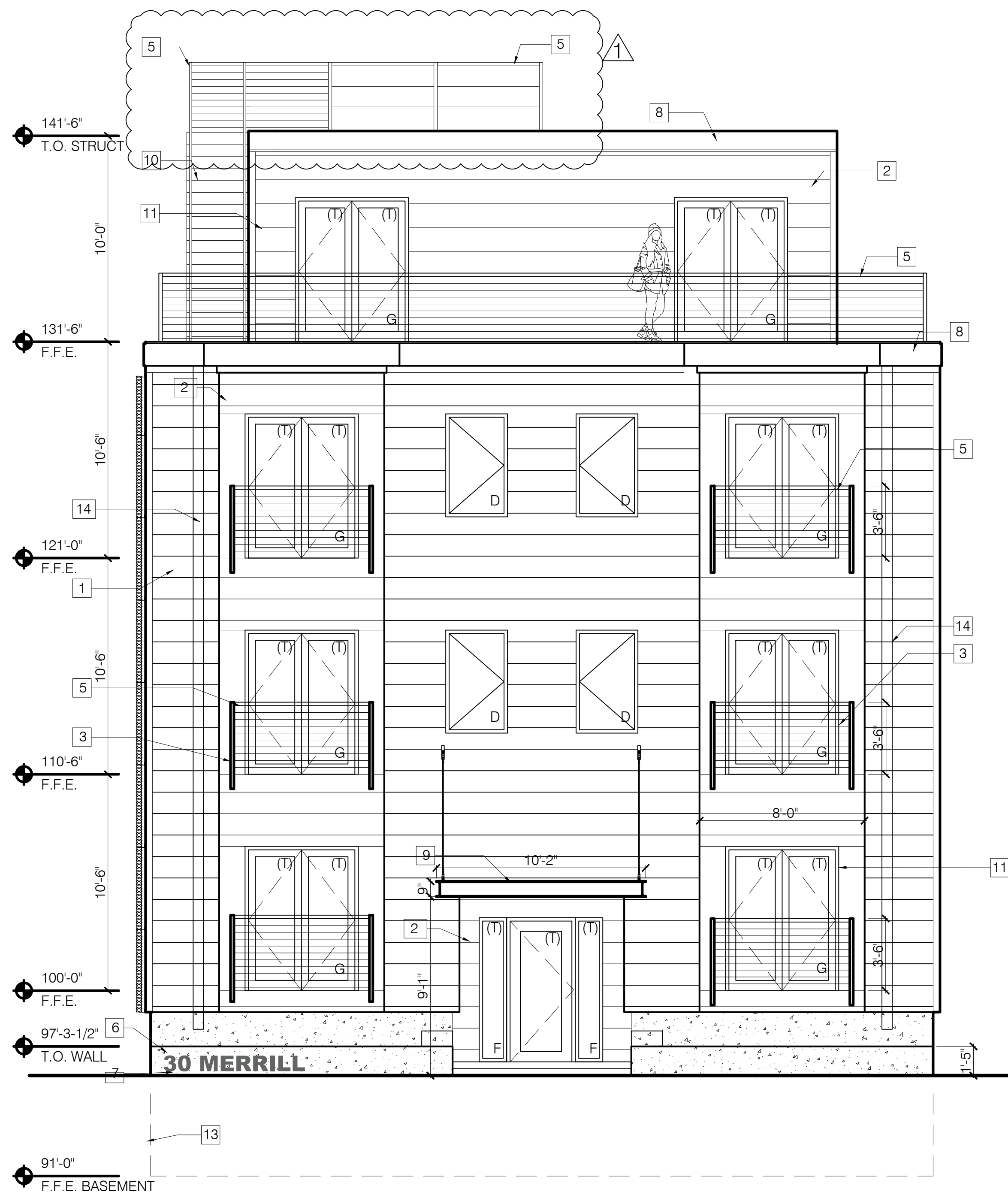
1 FRONT (EAST) ELEVATION SCALE: 1/4" = 1'-0"
