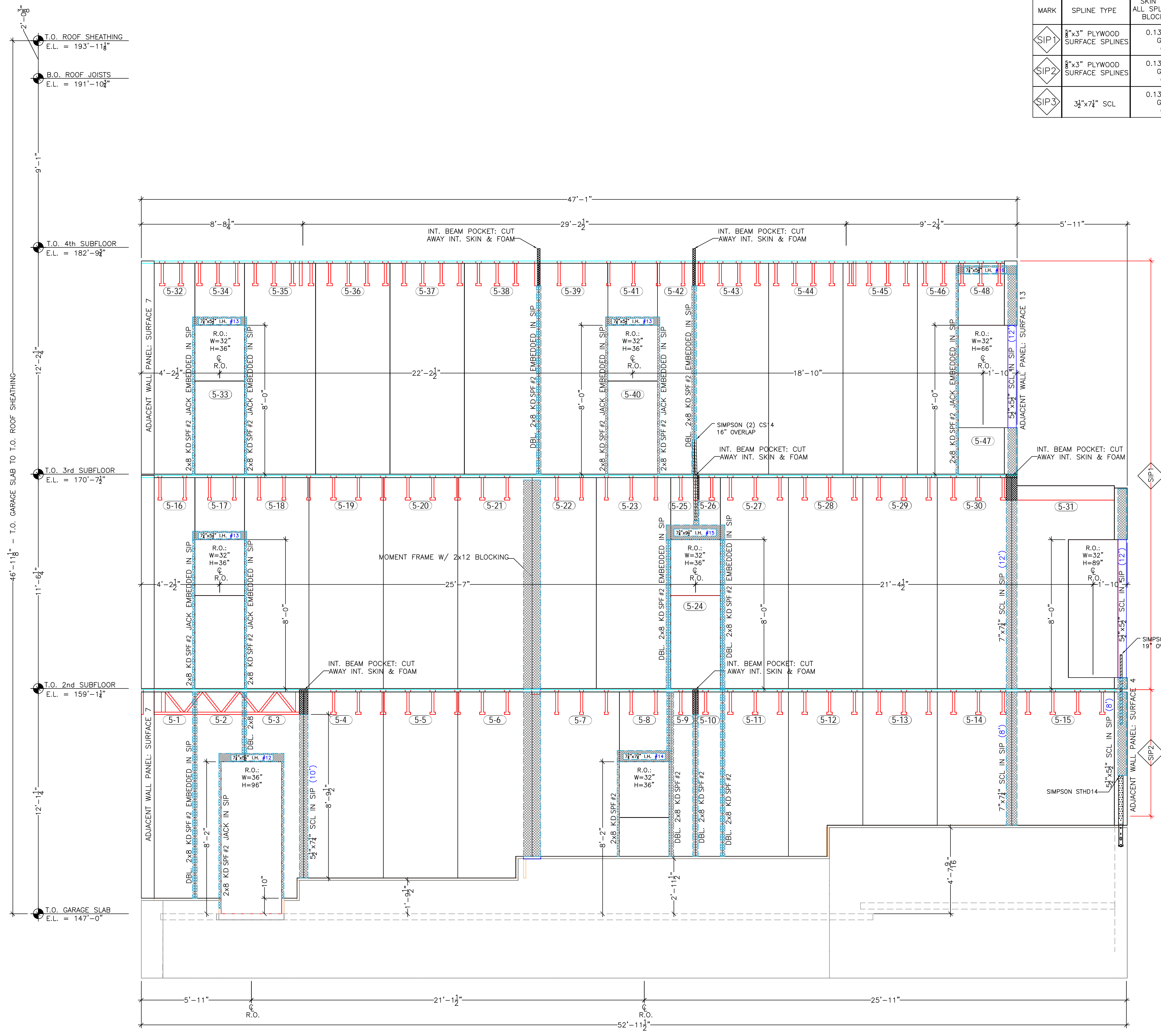
WALL PANEL LAYOUT: SURFACE 5 SCALE: 3/8" = 1'-0" PANEL_SPEC: 84" EPS SIP
