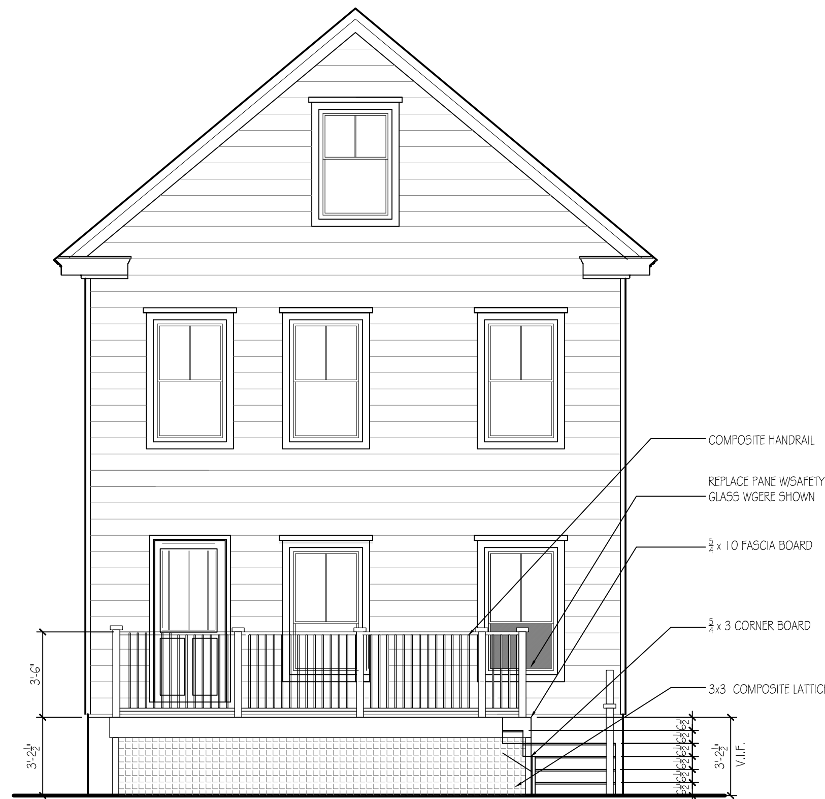
NEW DECK ELEVATION SCALE: 1/4" = 1'-0"
