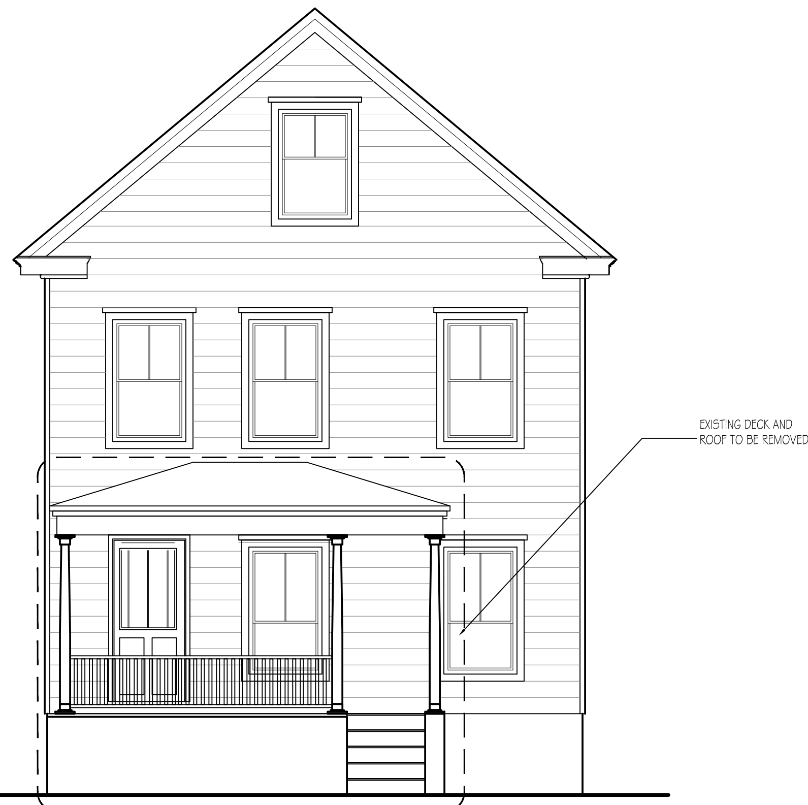
EXISTING DECK ELEVATION SCALE: 1/4" = 1'-0"
