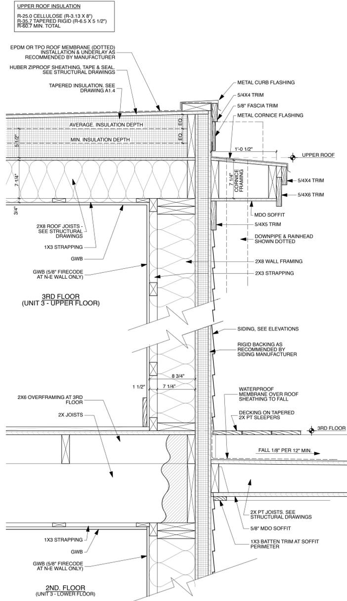
3 Wall section: 3rd floor, deck, upper roof - typical
