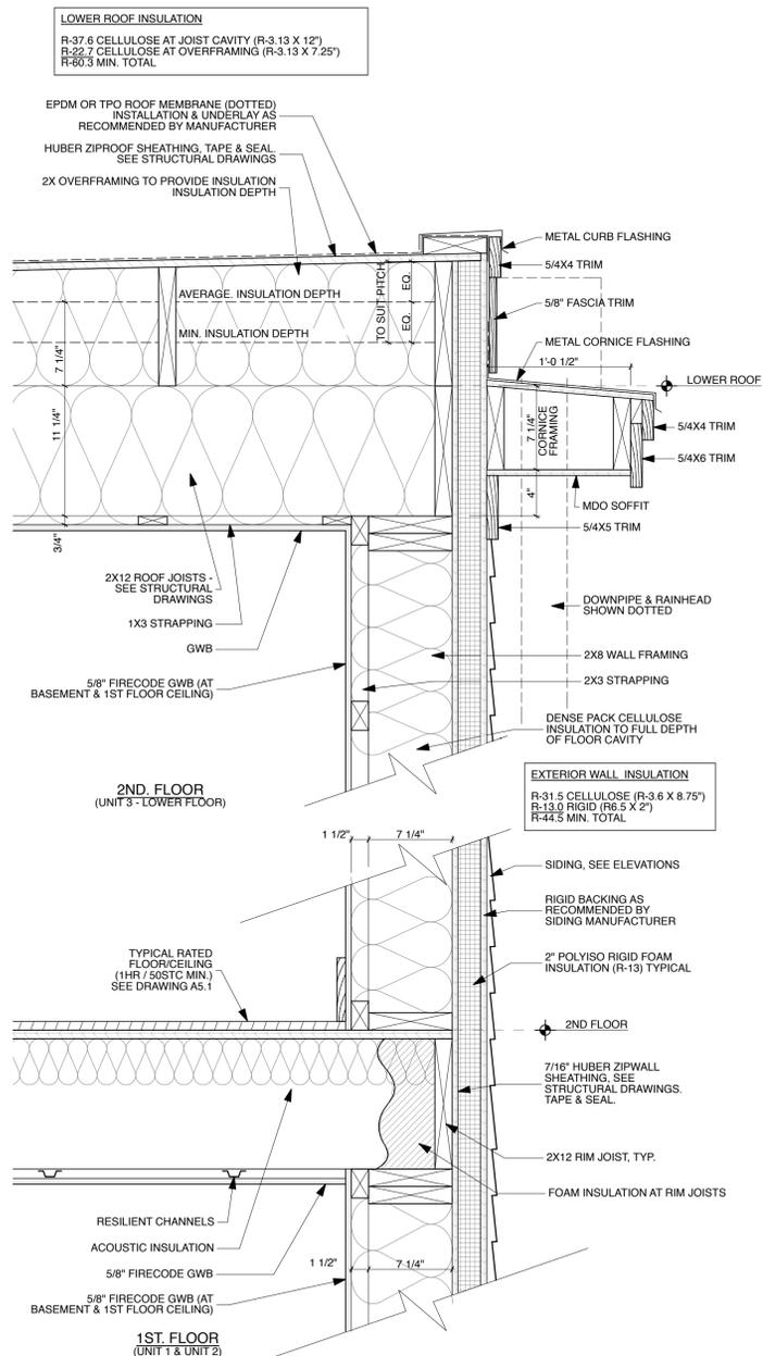
2 Wall section: 1st floor, 2nd. floor, lower roof - typ.
