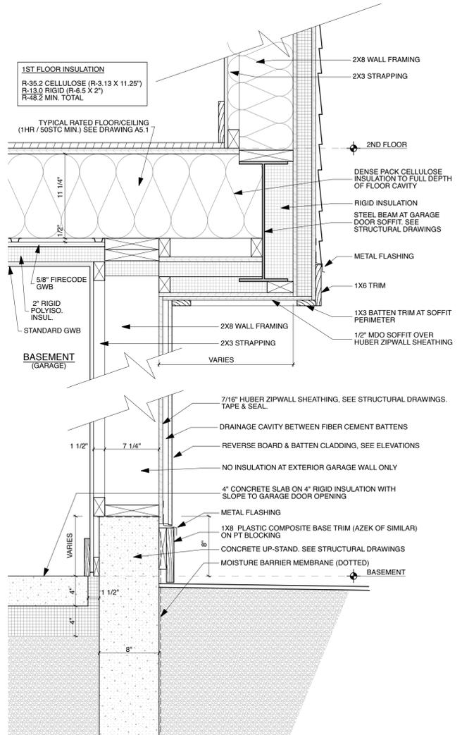
1 Wall section: Basement & exterior soffit - typical
