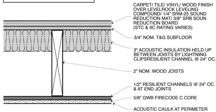
**4** Floor/ceiling: Min. 1-HR Fire / 50-STC / 50-IIC rating
