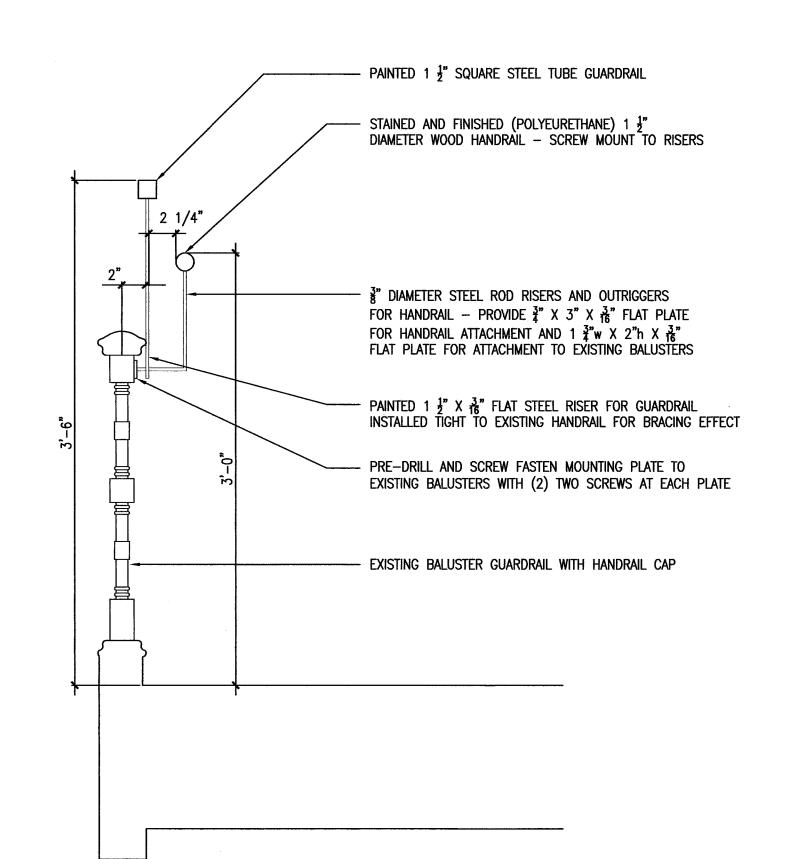
SECTION DETAIL AT NEW GUARDRAIL ASSEMBLY
