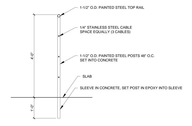
GUARDRAIL SECTION DETAIL SCALE 3/4" = 1'-0"
