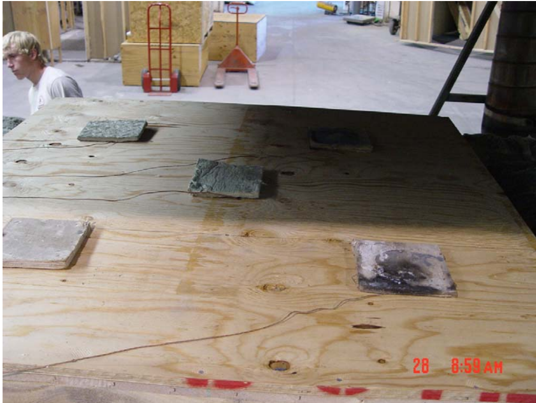
Photograph 3: Unexposed sample face pre-test showing thermocouple placement
