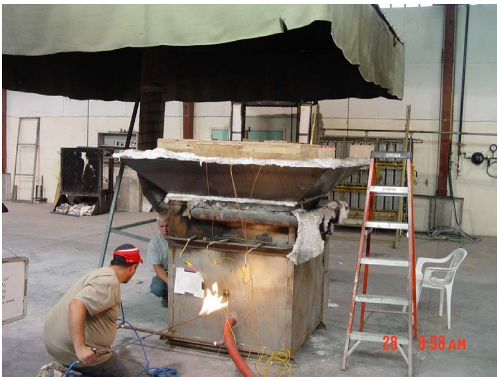
Photograph 2: Sample mounted on horizontal furnace at start of test
