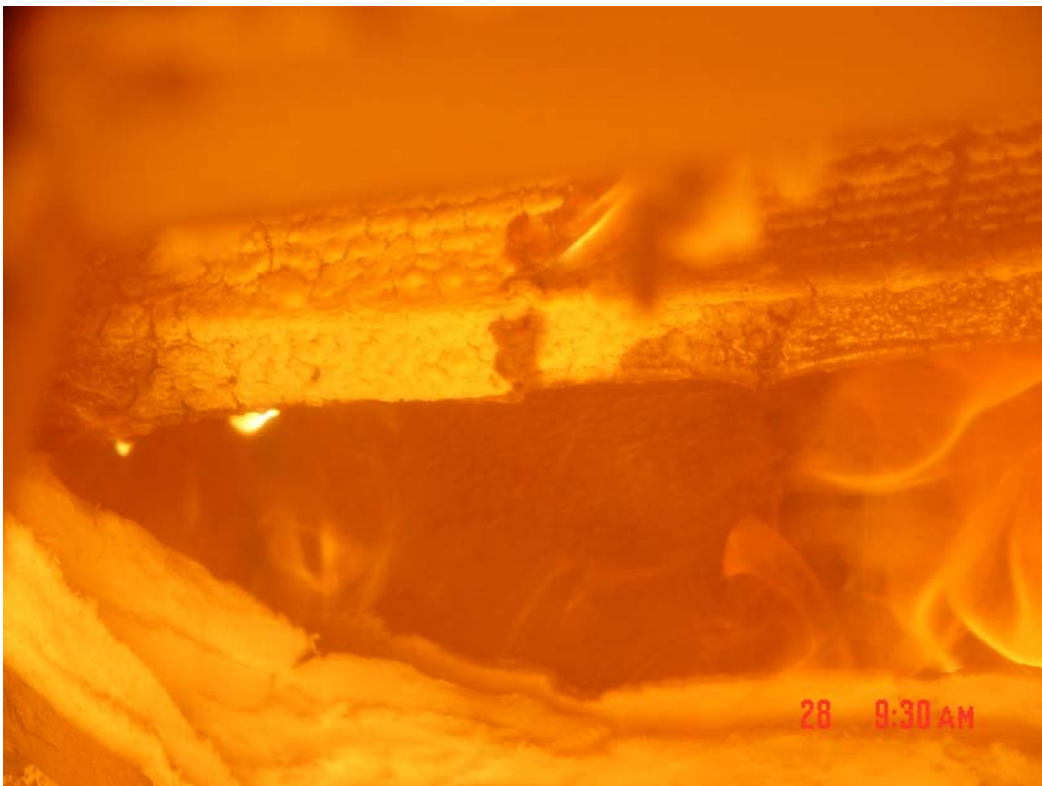
Photograph 8: Flame attaching to the sample during the test
