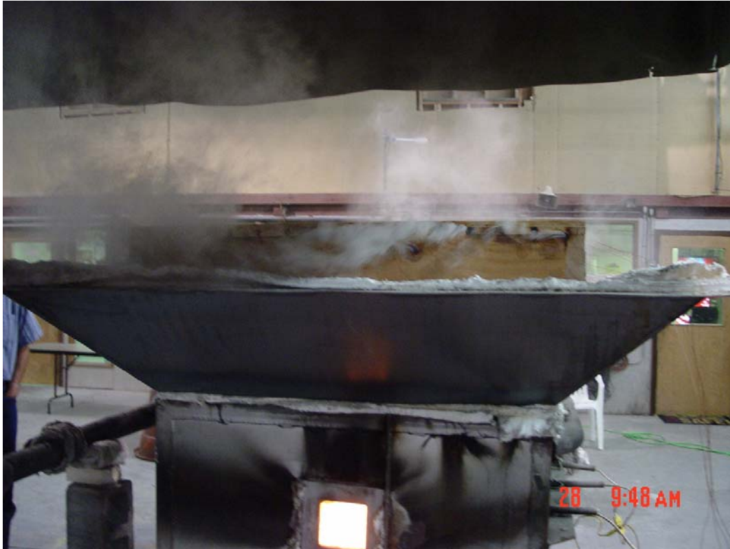
Photograph 9: Smoke rising from the sample during the test
