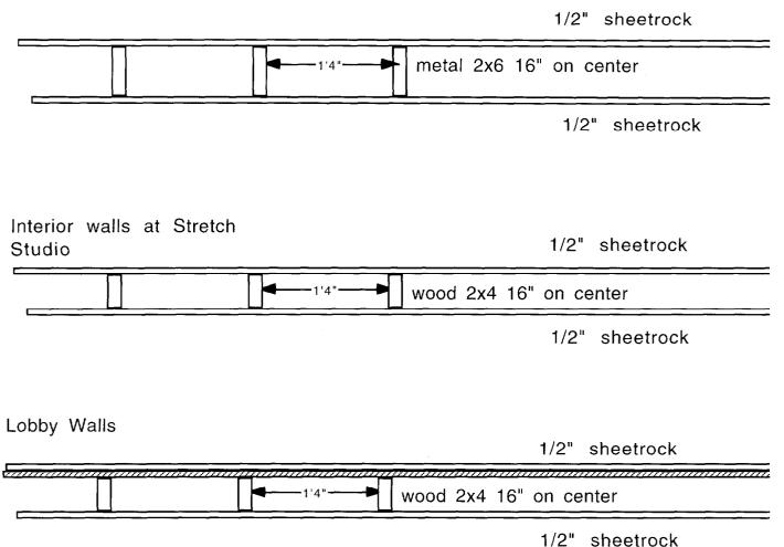
Lobby and shared room will have a storage loft floor above at 8' high. The joists will be wood 2x8s 16" on center and the deck will be 1/2 plywood.
