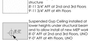
\_ Suspended Gyp Ceiling installed at lower heights under structural beams and to allow install of new MEP work 8'-0" AFF at 2nd and 3rd Floors, UNO 9'-0" AFF at 4th Floors, UNO
