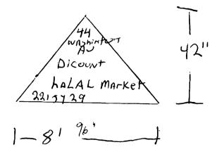
Sign will be Lag Bolted Into plywood & studs
