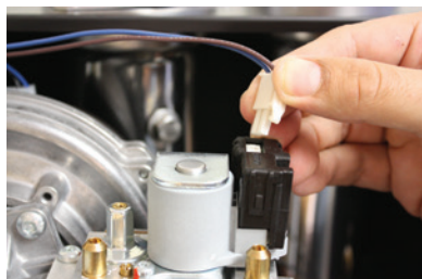
Disconnect gas valve harness plug
