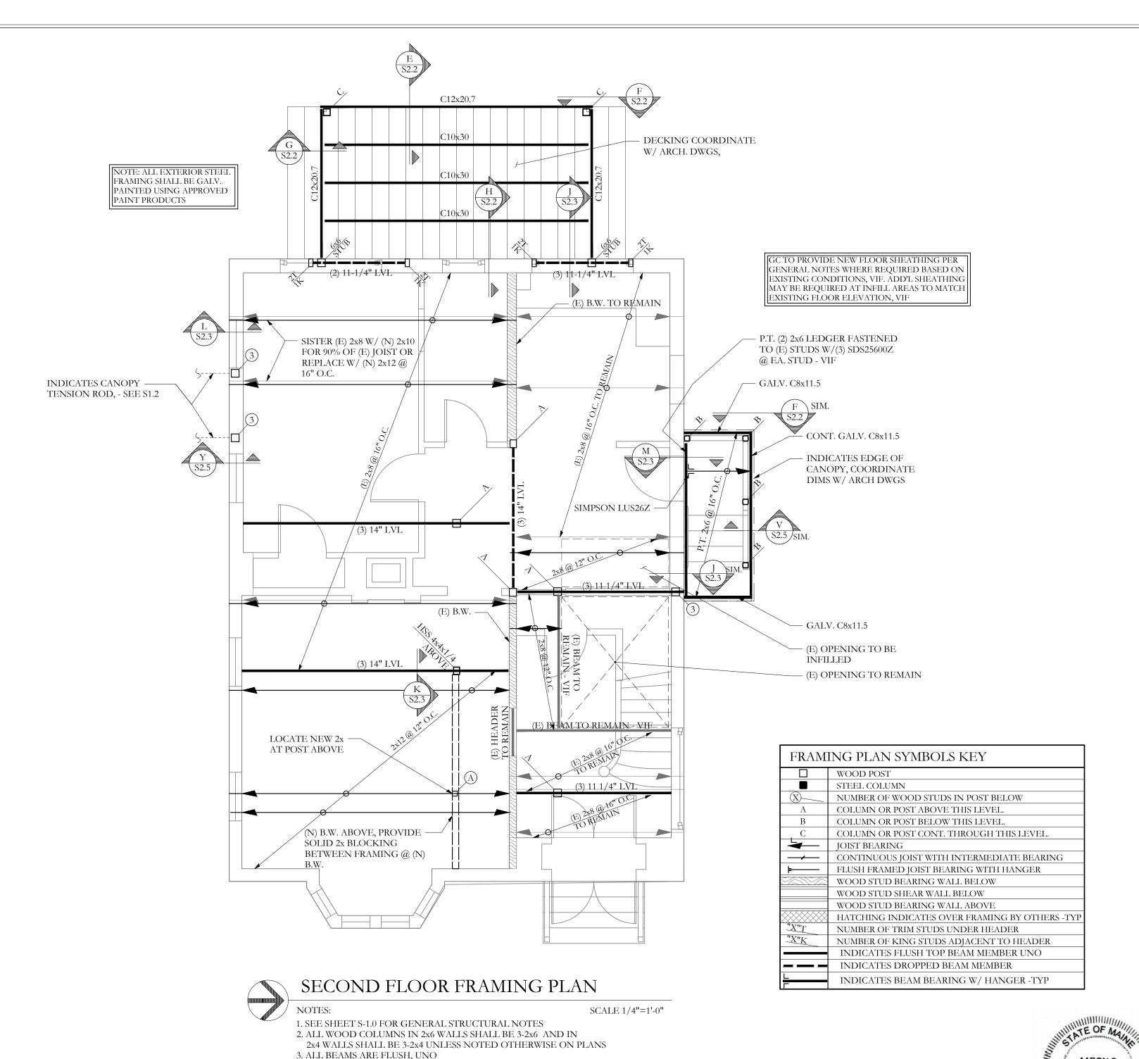
4. ALL HEADERS IN INTERIOR 2x BEARING WALLS ARE 2-2x6, UNO 5. ALL HEADERS IN EXTERIOR 2x BEARING WALLS ARE 3-2x6, UNO 6. FLOOR SHEATHING TO BE 3/4" T+G, SEE GENERAL NOTES FOR
