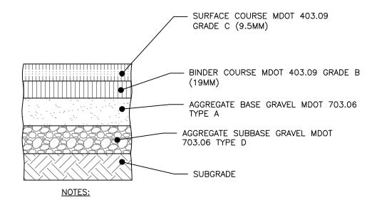
COMPACT SUBGRADE TO 95% MAXIMUM DRY DENSITY IN ACCORDANCE WITH ASTM D-1557.
