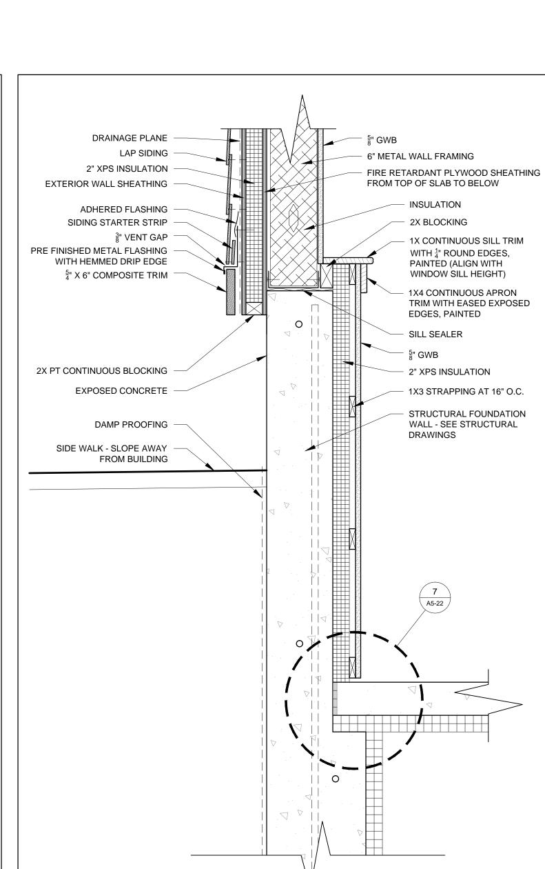
SECTION DETAIL AT FOUNDATION WALL IN GARAGE (SIDEWALK SIDE)
