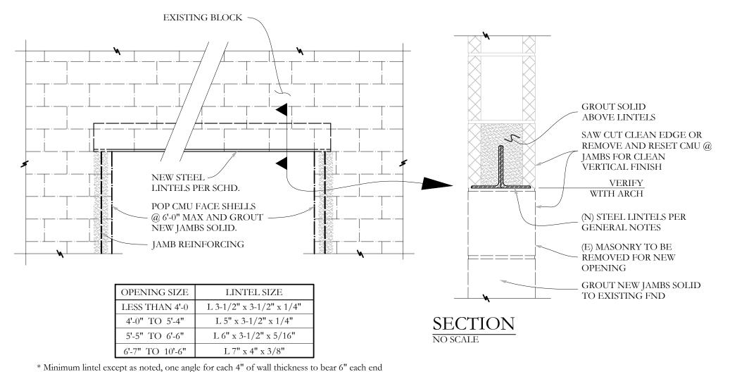
TYPICAL LOOSE LINTEL INSTALLATION IN EXISTING CMU NO SCALE
