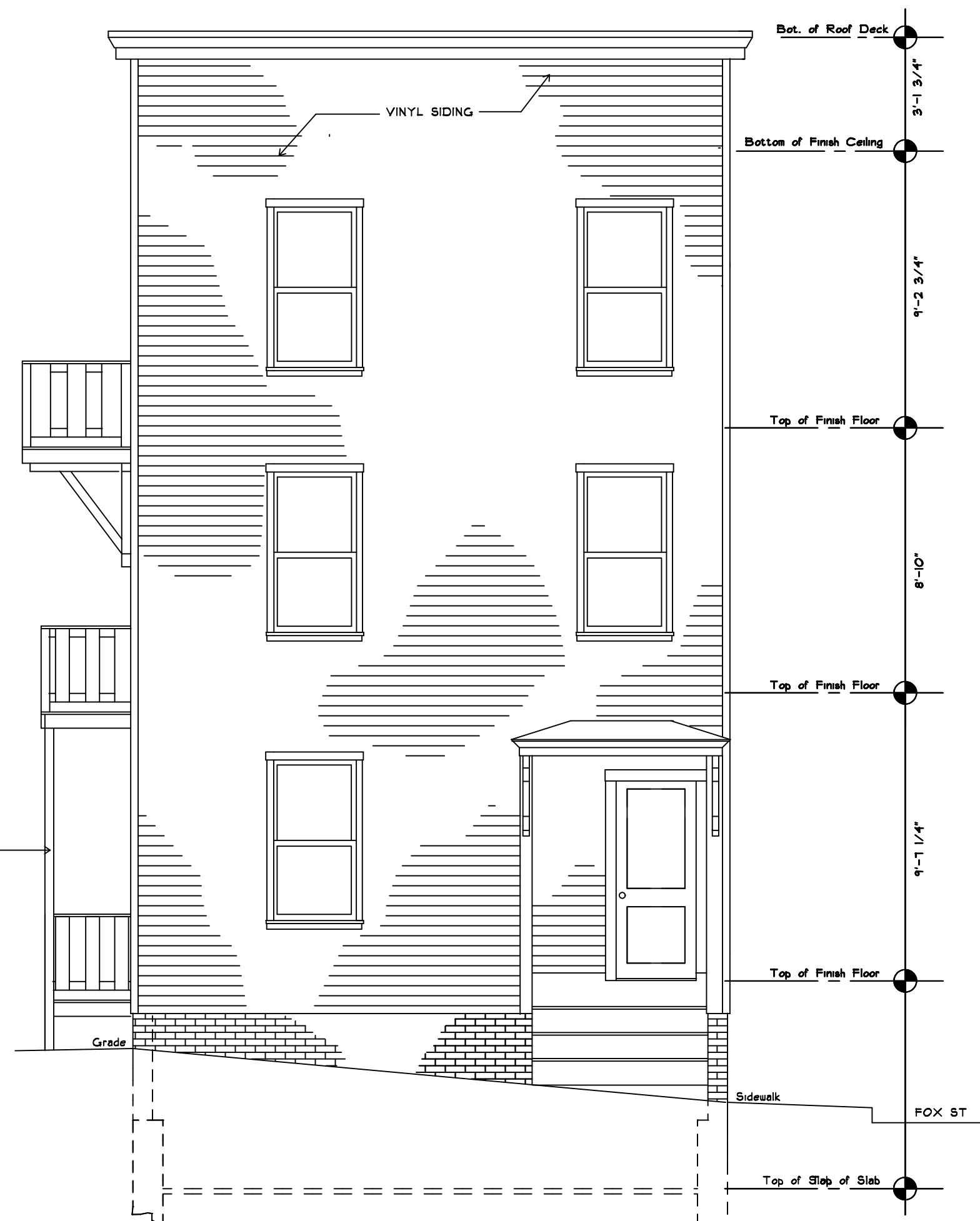
42 Greenleaf Street North Elevation 1/4"=1'-0"
