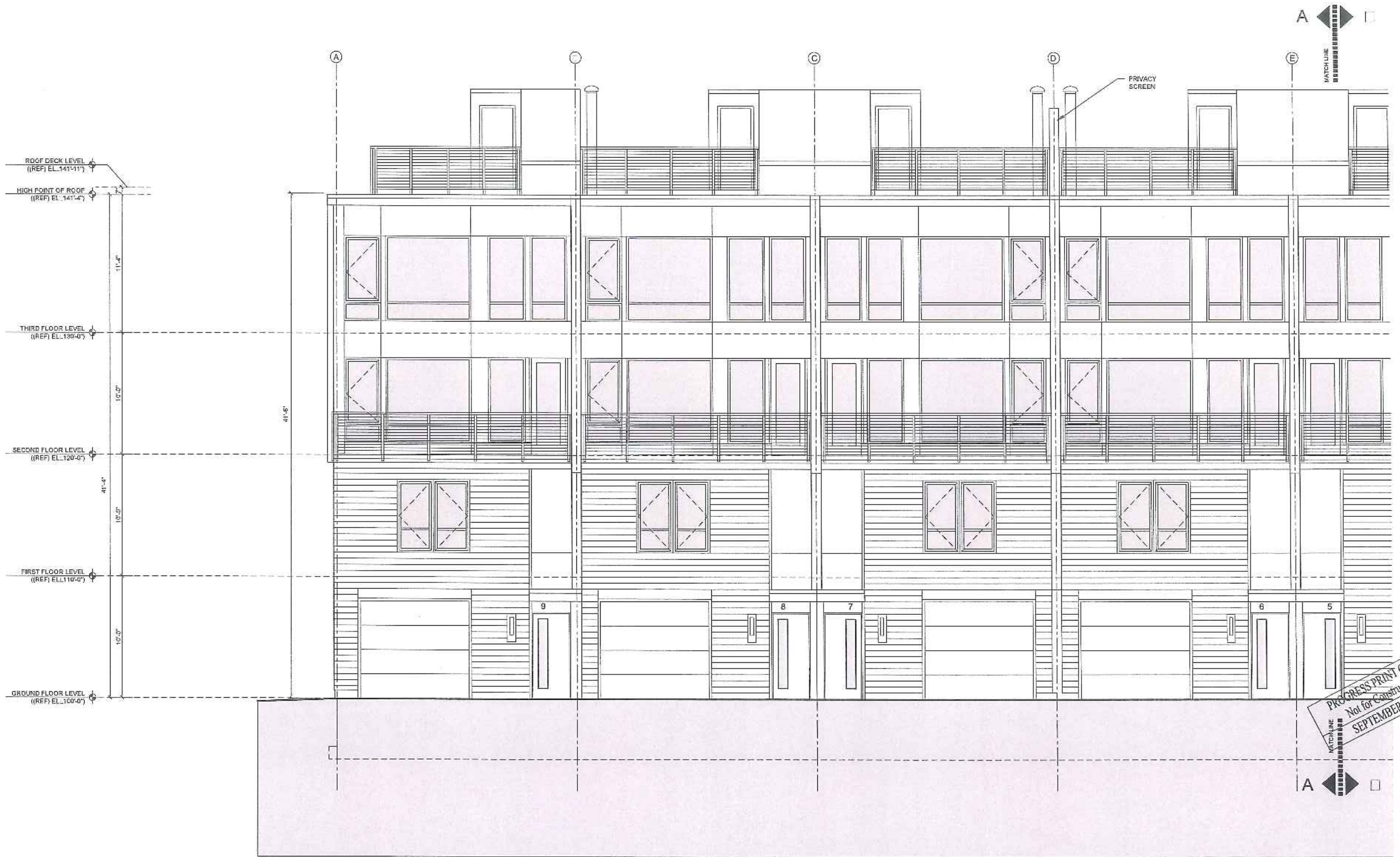
1 SOUTH ELEVATION - PART A 10'-1/4"
