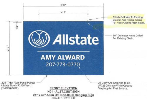
NOTE: All Dimensions And Field Conditions To Be Verified And Confirmed From Site Survey Prior To Releasing For Fabrication.
