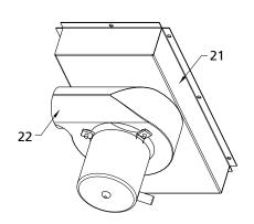
Figure 15 - Power Ventor Assembly (100/250 Unit Sizes Shown)
