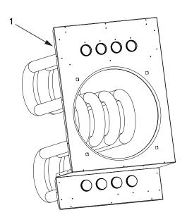
Figure 11 - Heat Exchanger Assembly
