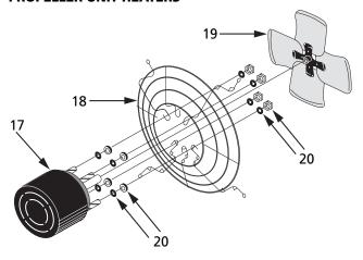
Figure 14 - Propeller Parts
