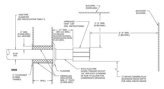
Figure 9A - Horizontal Arrangement - Single Wall Vent System to Single Wall Termination
