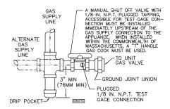
Figure 4 - Pipe Installation, Standard **Controls**
