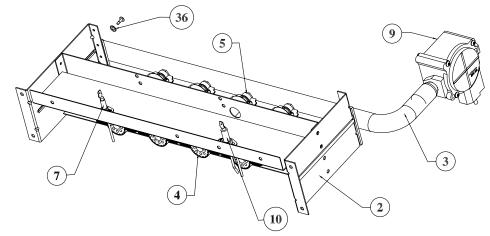
Figure 13 - Manifold Burner Assembly
