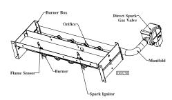
Figure 10 - Manifold Assembly
