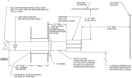
Figure 8A - Horizontal Arrangement - Single Wall Vent System to Double Wall Termination
