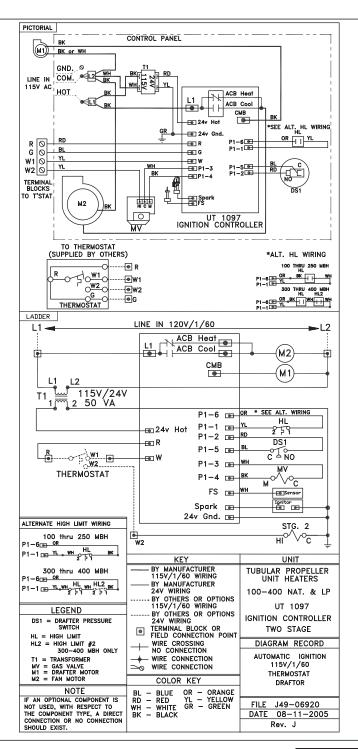
Figure 5C- Tubular Units Equipped with Optional 2 Stage Ignition Natural Gas and Propane (LP) Gas
