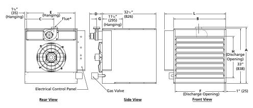
(\*) For all installations, the flue collar is included with the unit and should be field installed per the instructions included – see Figure 3A.
