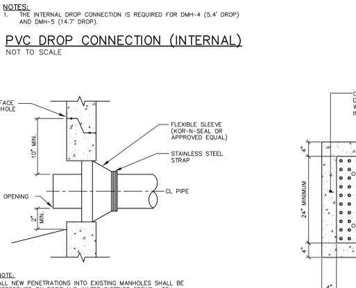
**NEW PIPE TO EXISTING MANHOLE CONNECTION - 4" TO 24"**
