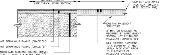
**PAVEMENT SAW CUT DETAIL**
