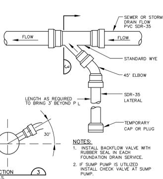
**SEWER / FOUNDATION DRAIN SERVICE CONNECTION**
