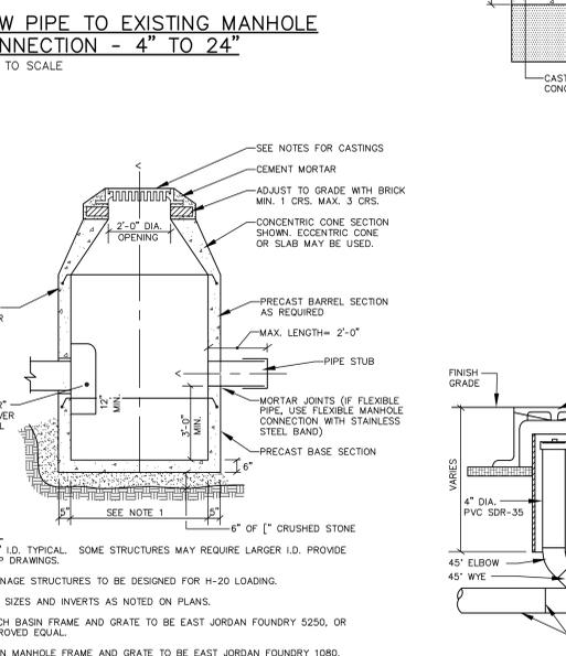
**TYPICAL DRAINAGE MANHOLE/CATCH BASIN**
