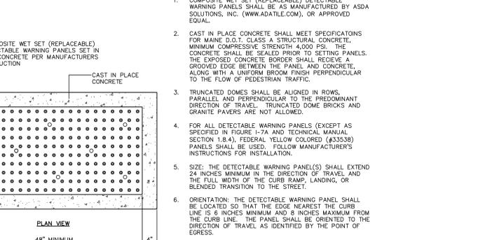
**SIDEWALK RAMP DETECTABLE WARNING PANEL**
