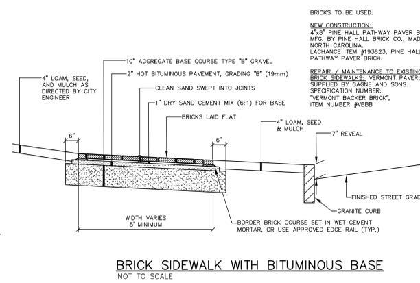
**BRICK SIDEWALK WITH BITUMINOUS BASE**
