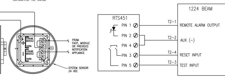
CEILING HORN/STROBE WIRING DETAIL SCHEMATIC: NO SCALE
