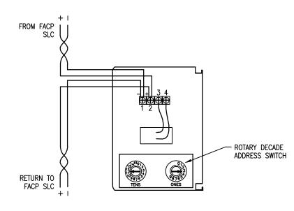
MANUAL PULL STATION WIRING DETAIL SCHEMATIC: NO SCALE
