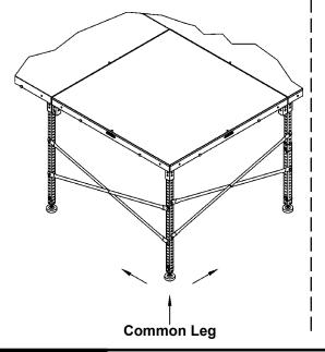
E. Multi-Stage should be braced every 2-3 decks as shown when bracing is required. (Note the common leg bracing method is shown below.)
