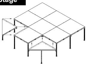
When a 45° stage is mated to the notched side of a deck, bolting is required using:
