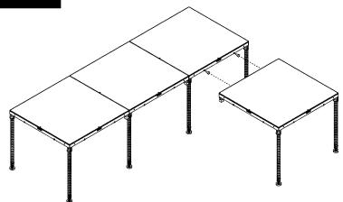
Upon completion of the back row, begin the second row with one section and two legs as shown in Step 4- B, C & D.
