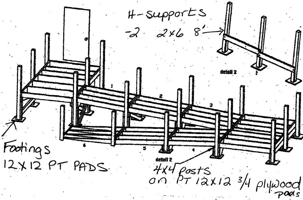
Note: The same options for transition to the ground are used for this design. Guardrail/handrail options are also the same except the inside guardrail on the lower portion of the ramp will be attached to the center 4x4's. Between modules 3 & 4 some 2x2x30's spindles will need to be screwed in place from inside the ramp.
