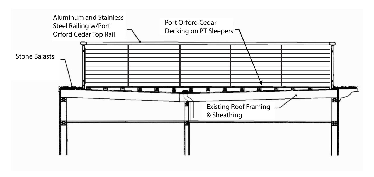
SECTION THROUGH ROOF DECK
