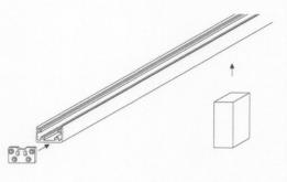
c. Locate crush block(s) provided to the bottom Aluminum Rail Reinforcement, with spacing no greater than 36" from the end, or between Crush Blocks.
