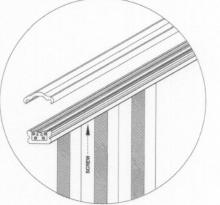
e. Drill a 3/16" hole through the aluminum reinforcement over every third baluster (note: offset to avoid the screw which attaches the Baluster to the Top Common Rail) and secure the aluminum reinforcement to the rail/baluster assembly using *baluster screws* (E)
